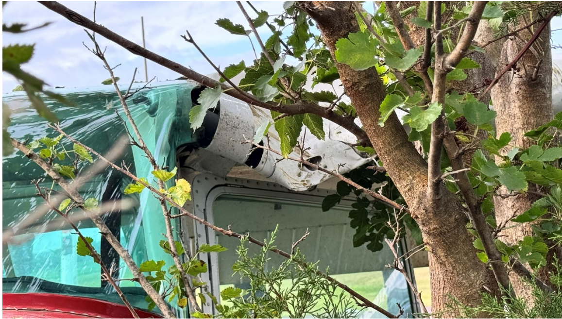
Photograph 2 - Damage to left wing (Courtesy of FAA)
