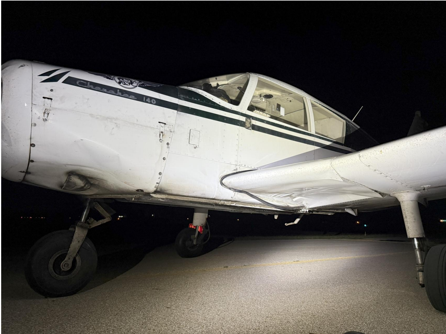
Photograph 1 - Airplane Damage Sustained During Deer Strike (Courtesy of Pilot)
