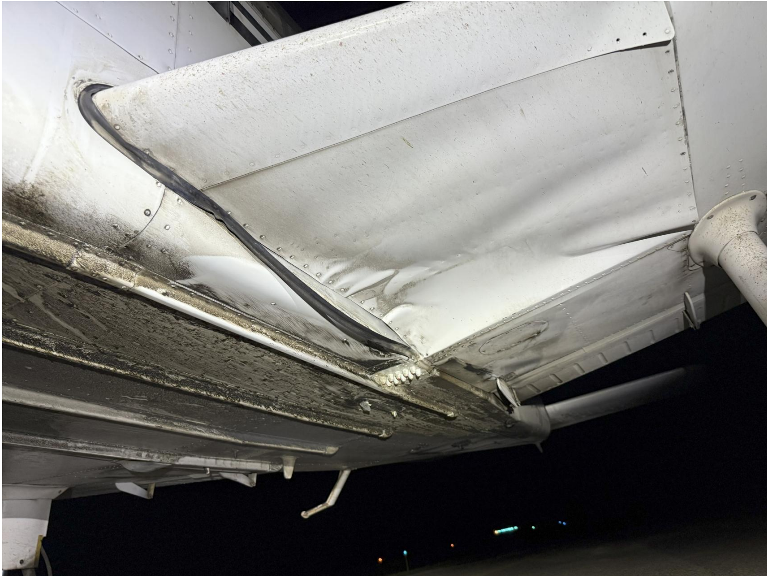
Photograph 2 - Left Wing Damage (Courtesy of Pilot)
