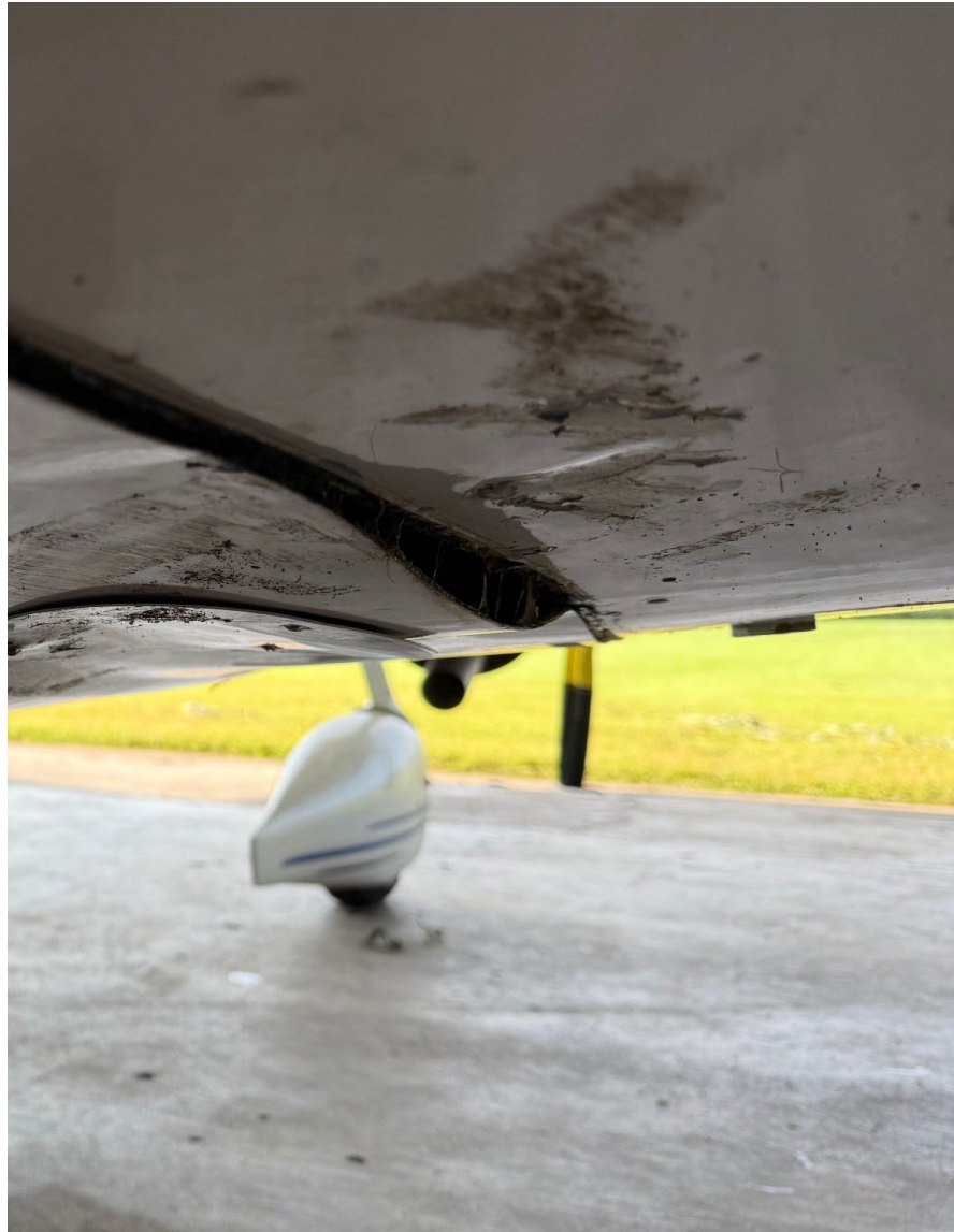
Photograph 2 - Wing Damage (Courtesy of Federal Aviation Administration)
