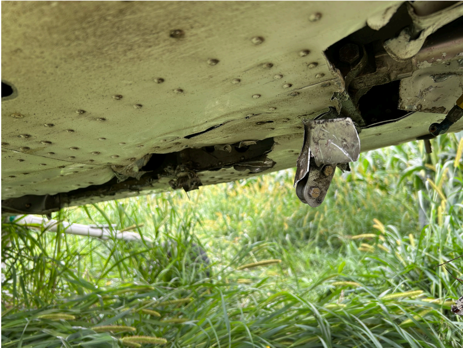
Photograph 2 - Lower Fuselage Substantial Damage (Courtesy of FAA)
