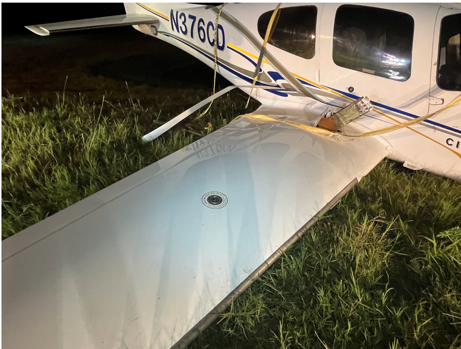
Photograph 2 - Right wing damage (Courtesy of FAA)
