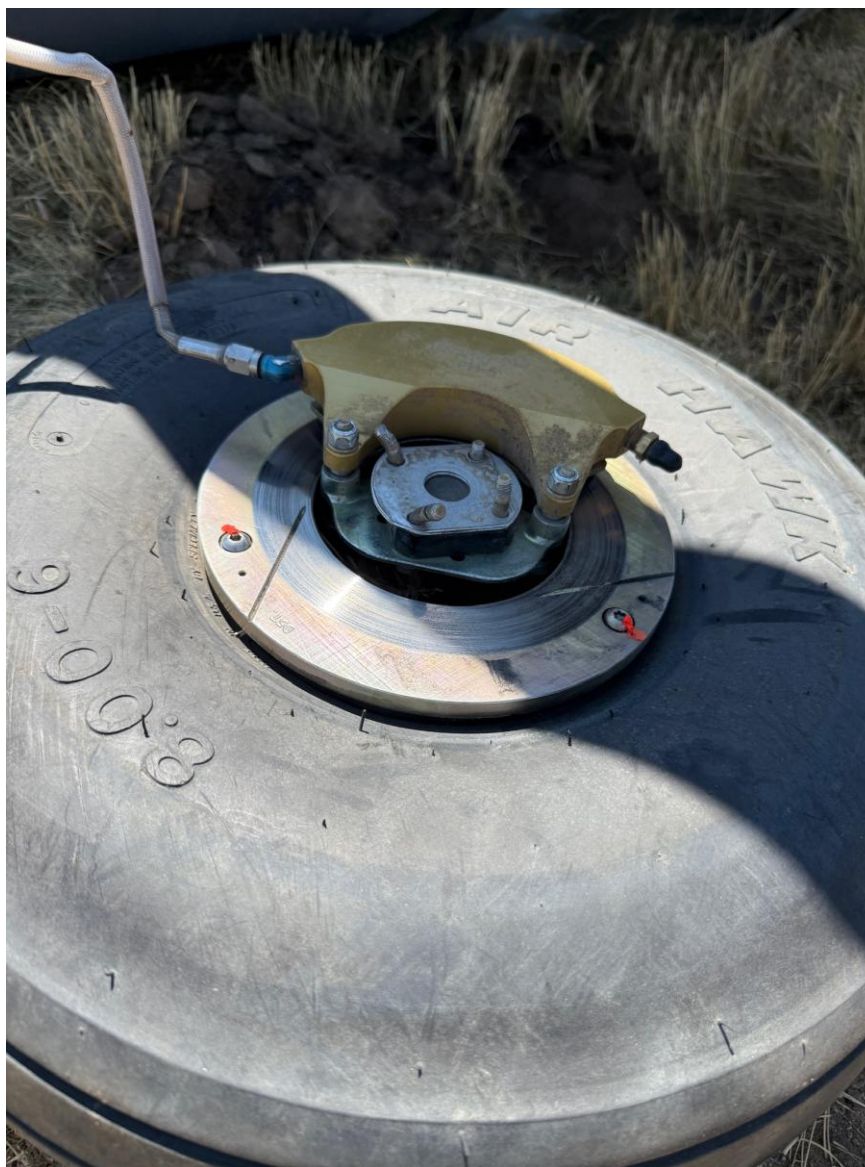
Photograph 5 - Separated wheel assembly (FAA photo)
