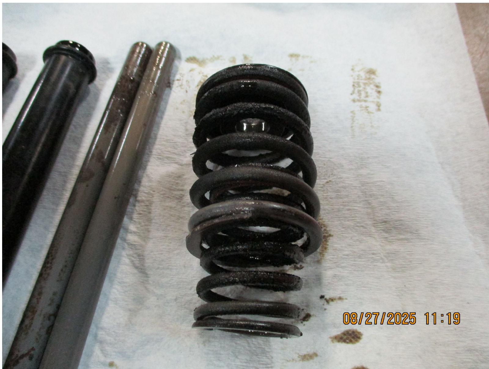
Photograph 10 - No. 2 exhaust valve springs and push rods (Courtesy of FAA)
