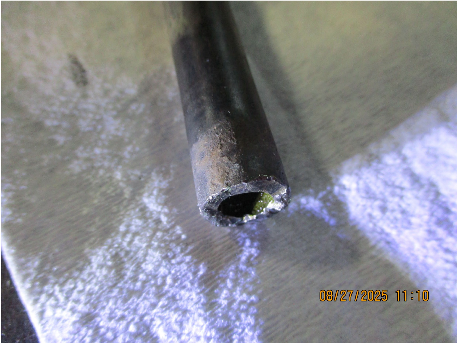
Photograph 9 - No. 2 exhaust valve stem (Courtesy of FAA)
