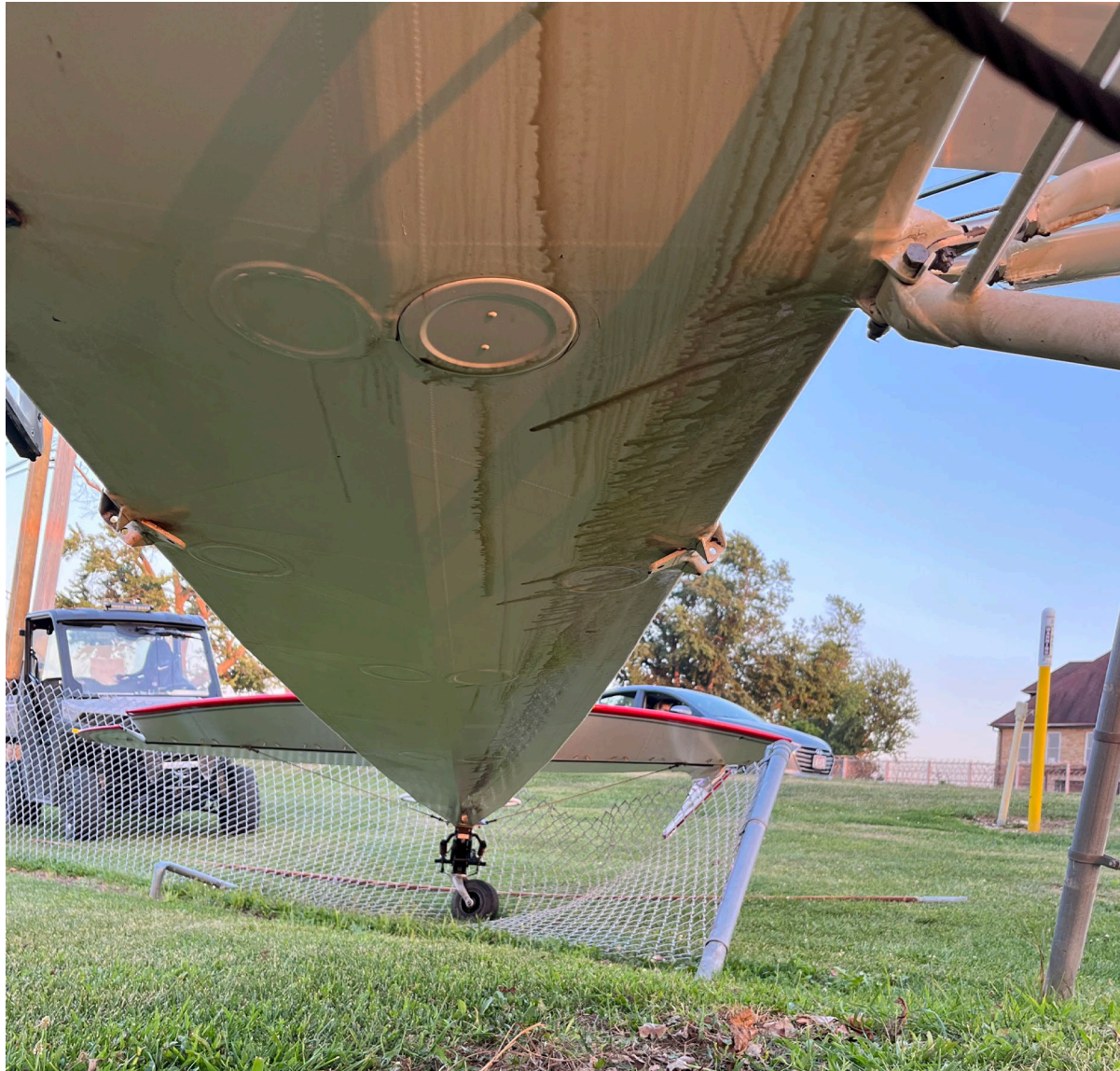
Photograph 2 - Oil under fuselage (Courtesy of FAA)
