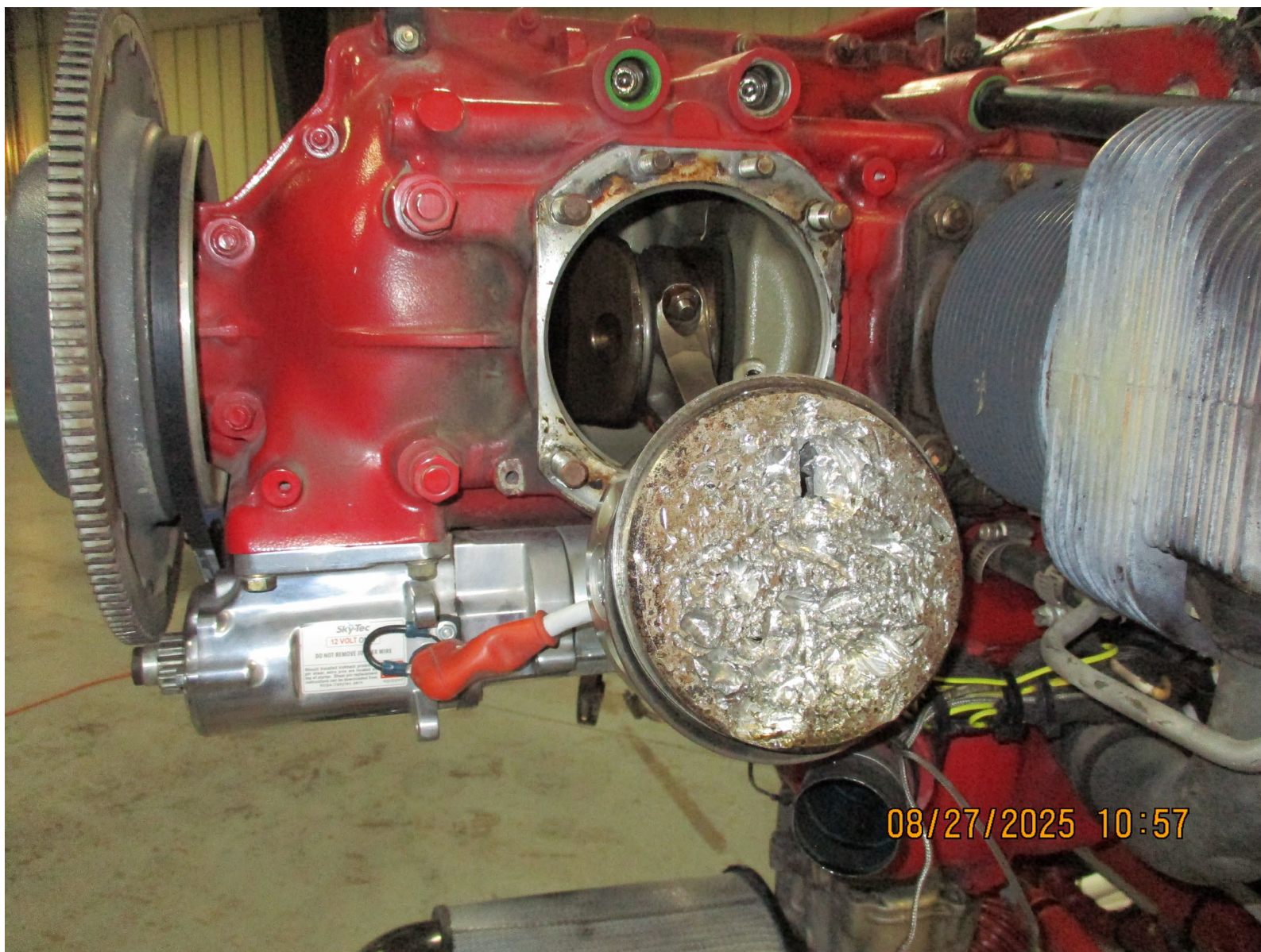
Photograph 4 - No. 2 piston (Courtesy of FAA)
