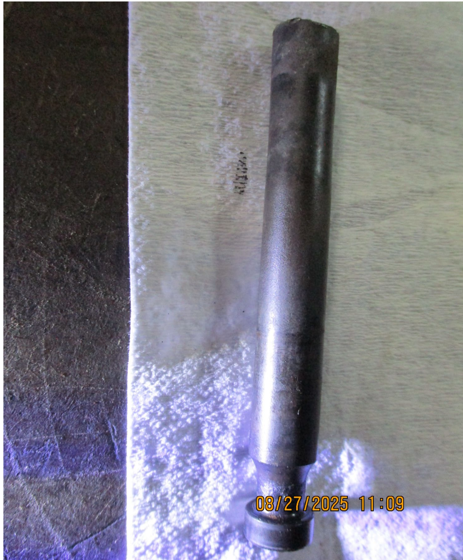
Photograph 8 - No. 2 exhaust valve stem (Courtesy of FAA)
