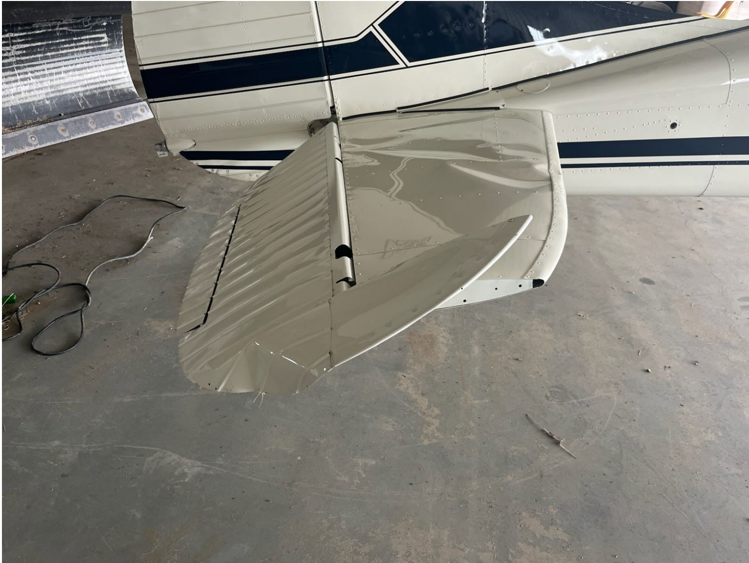
Photograph 2 - Right Horizontal Stabilizer Damage (Courtesy of Federal Aviation Administration)
