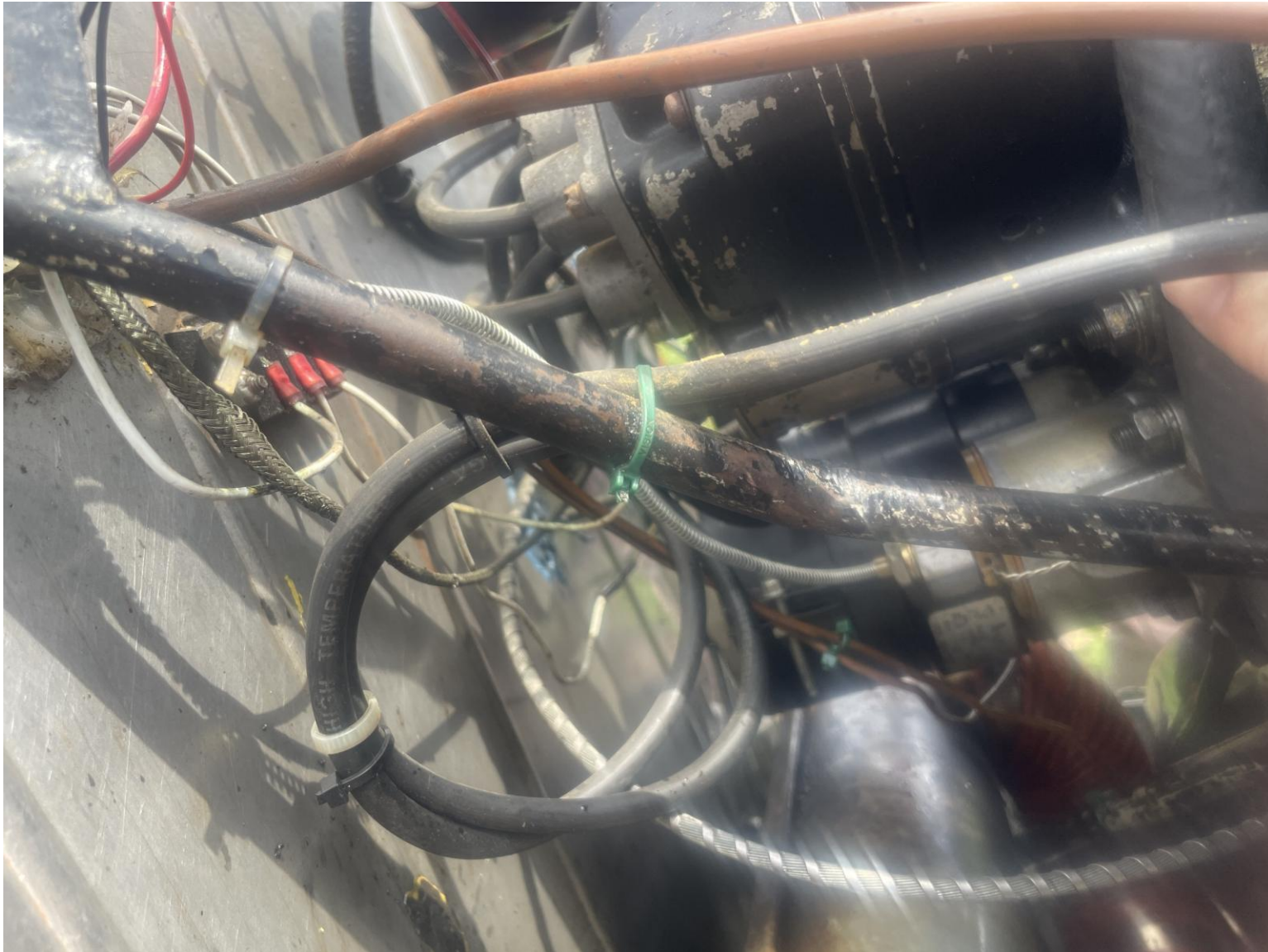
Photograph 3 - Engine mount tube damage (Courtesy of FAA)
