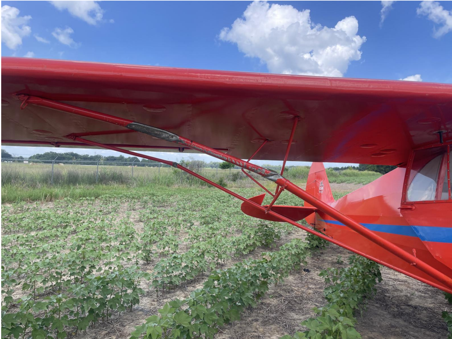
Photograph 2 - Right wing strut damage (Courtesy of FAA)
