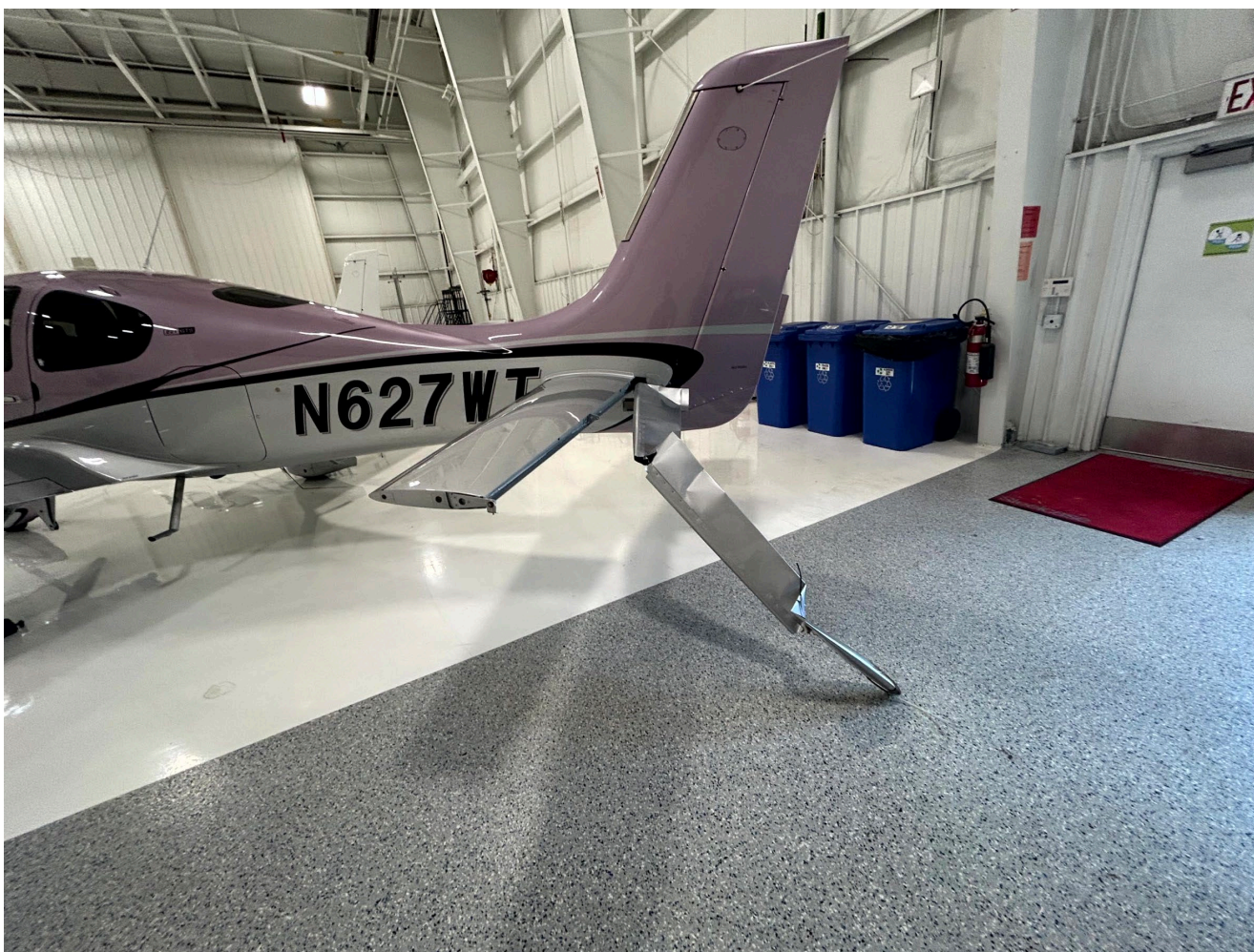
Photograph 1 - Left Elevator Damage (Courtesy of FAA)
