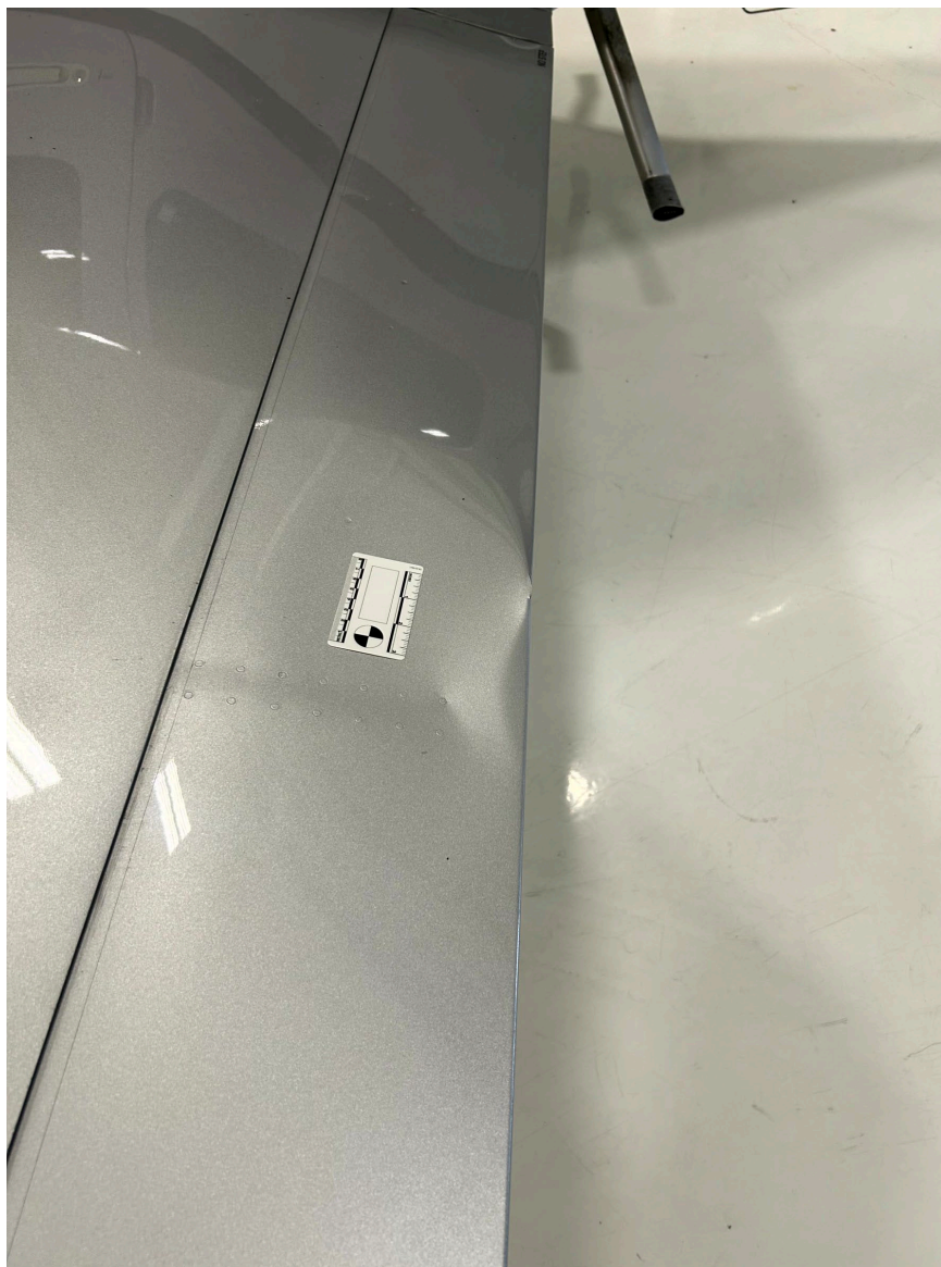
Photograph 2 - Left Flap Damage (Courtesy of FAA)
