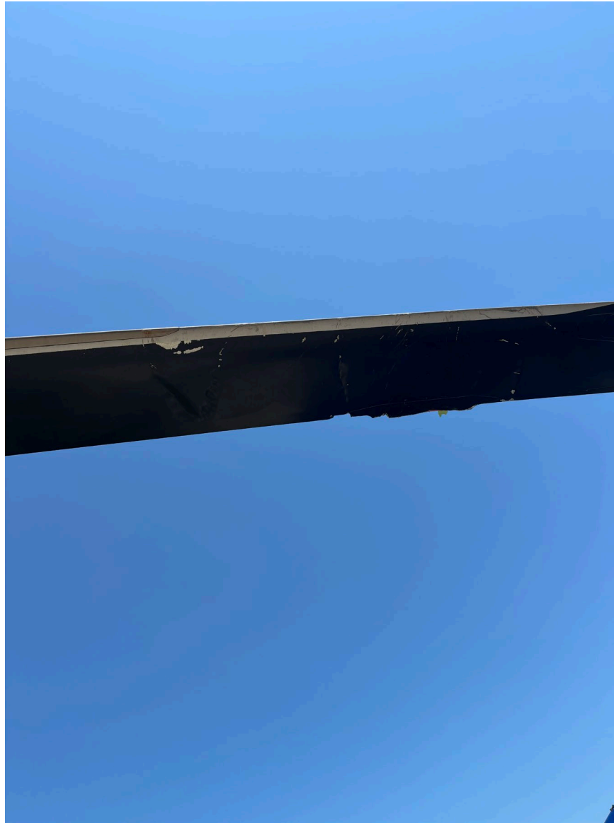
Photograph 1 - Damage to helicopter's main rotor blade (Courtesy of FAA)
