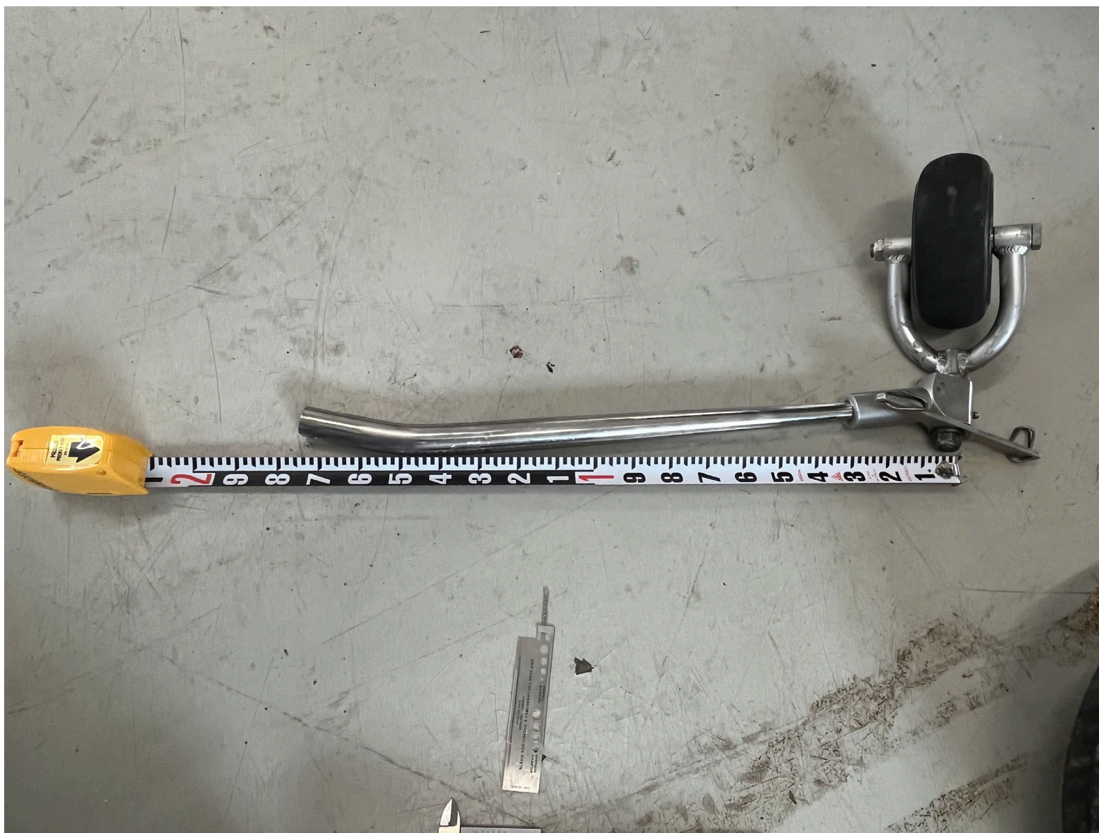
Photograph 4 - Tailspring and tailwheel assembly (Courtesy of FAA)
