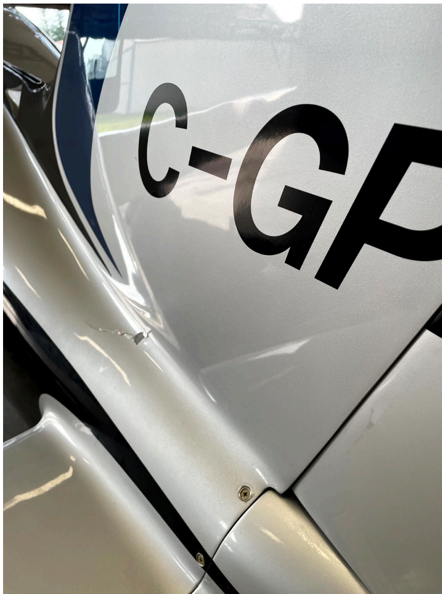
Photograph 3 - Damage at aft fuselage/empennage (Courtesy of FAA)
