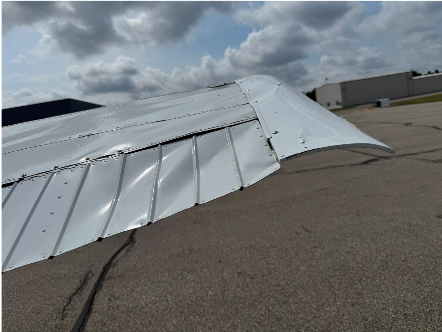
Photograph 2 - Right wing damage (Courtesy of pilot)
