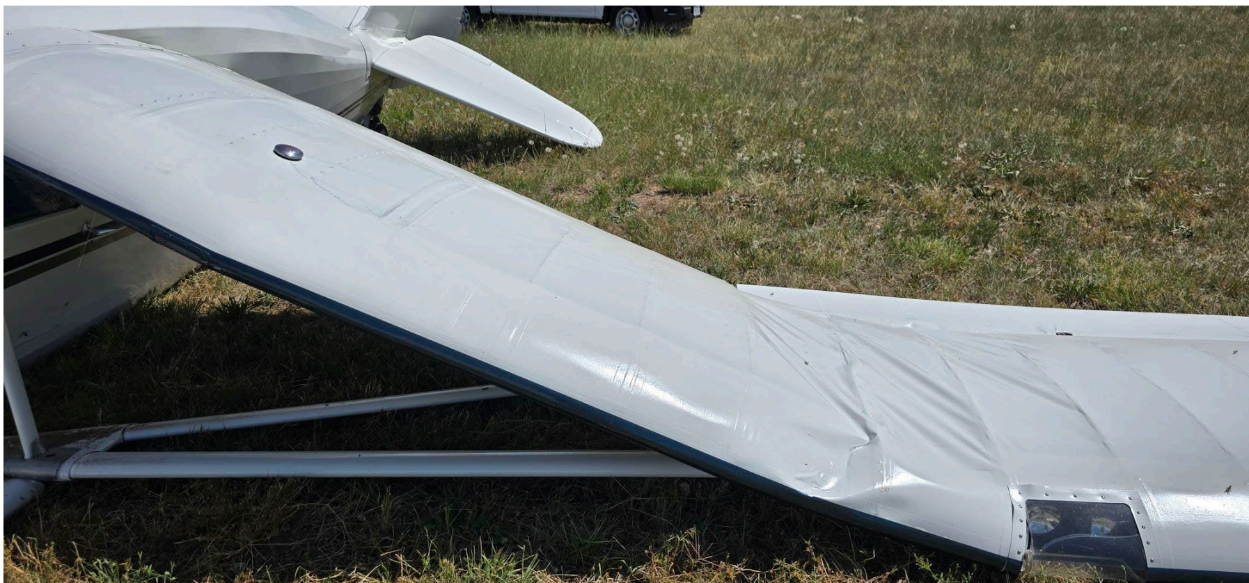
Photograph 1 - Wing Damage (Courtesy of Airfield Management)
