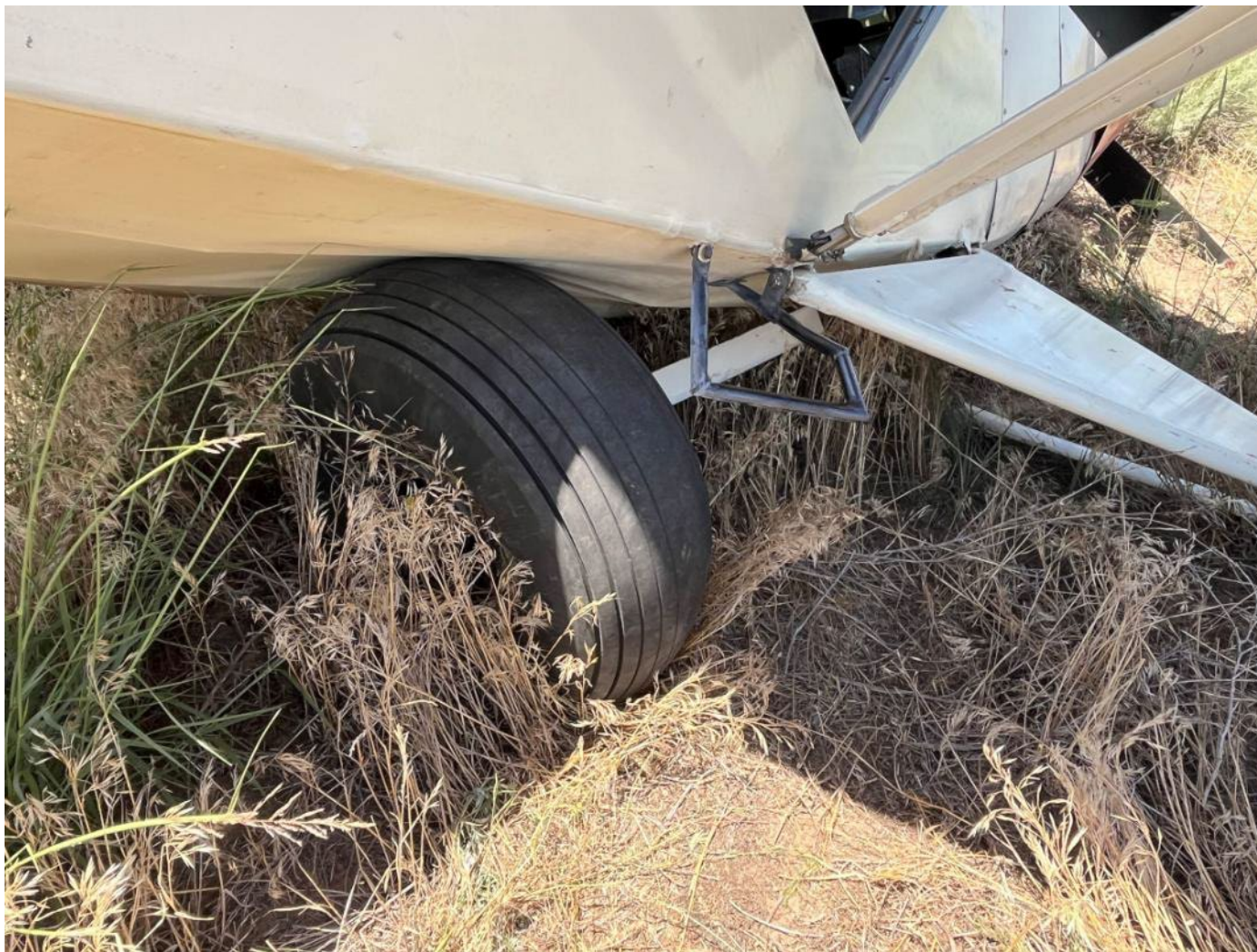
Photograph 2 - Fuselage Damage (Courtesy of Pilot)
