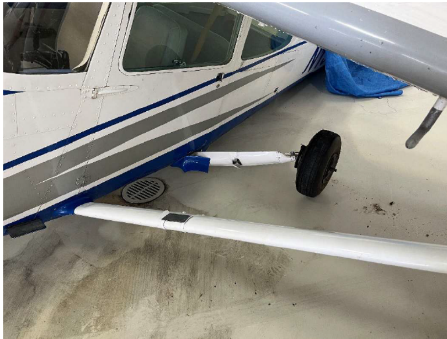
Left gear leg swept back due to the shearing of the gear leg attachment bolt.
