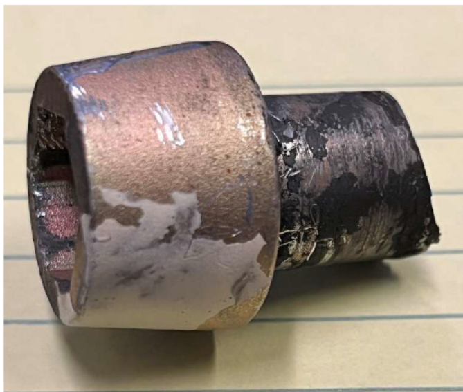
As removed bolt head. Note original Cessna factory witness paint. Metal shows signs of shear stress.
