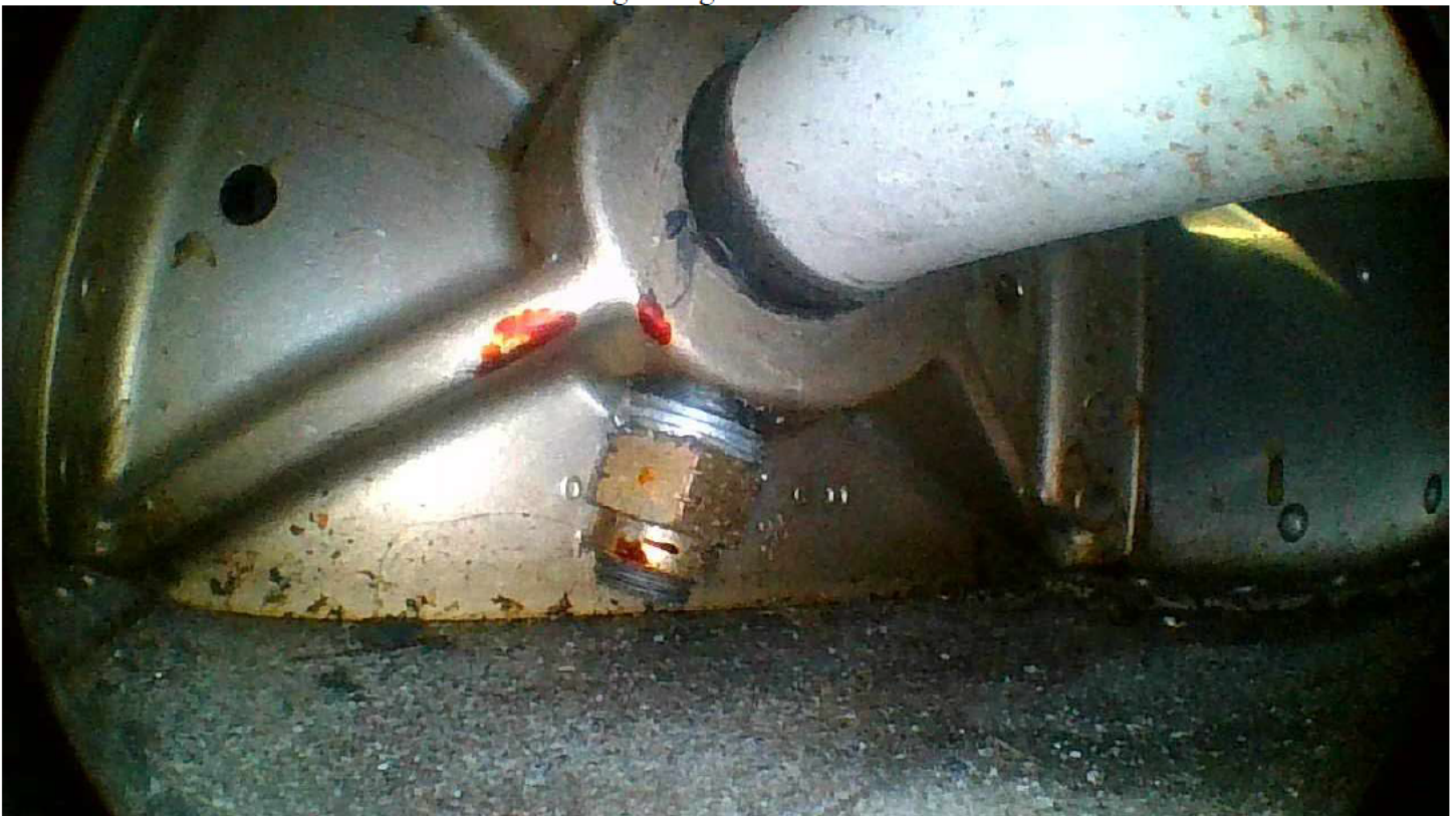
Nut end of the sheared left gear attach bolt.
