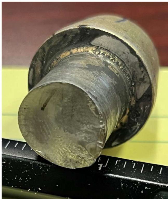
As removed bolt head. Note original Cessna factory witness paint. Metal shows signs of shear stress.
