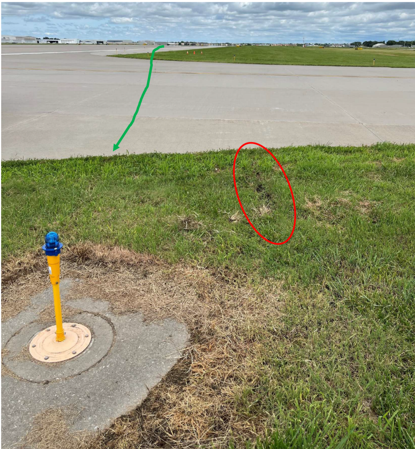
The green arrow parallels the right main tire mark. The red circle is a ground scar from the left main gear leg fairing. Blue taxiway light replaced due to impact with belly of aircraft.
