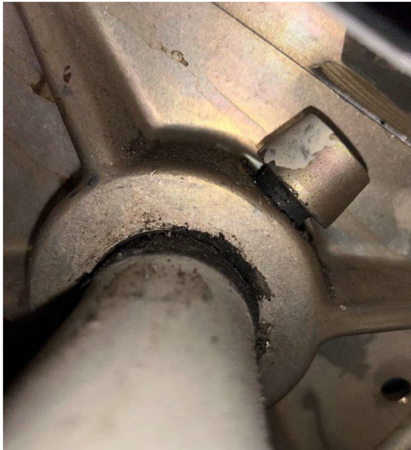
Left gear leg bolt as found.
