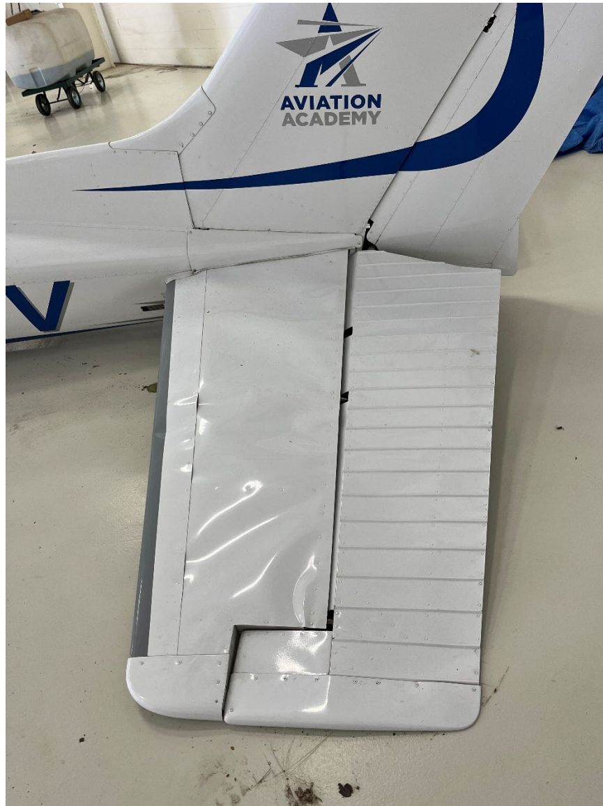
Photograph 5 - View of the substantial damage sustained to the left horizontal stabilizer (courtesy of the Federal Aviation Administration)
