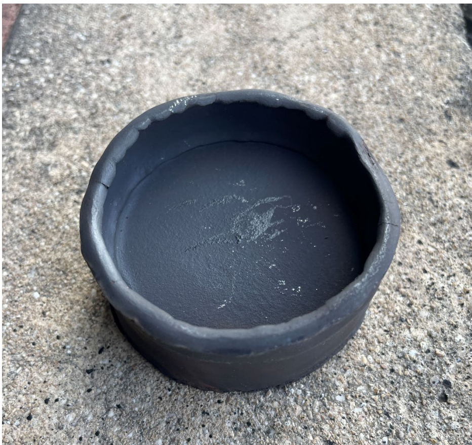
Figure 2. Obstruction removed from exhaust pipe.
