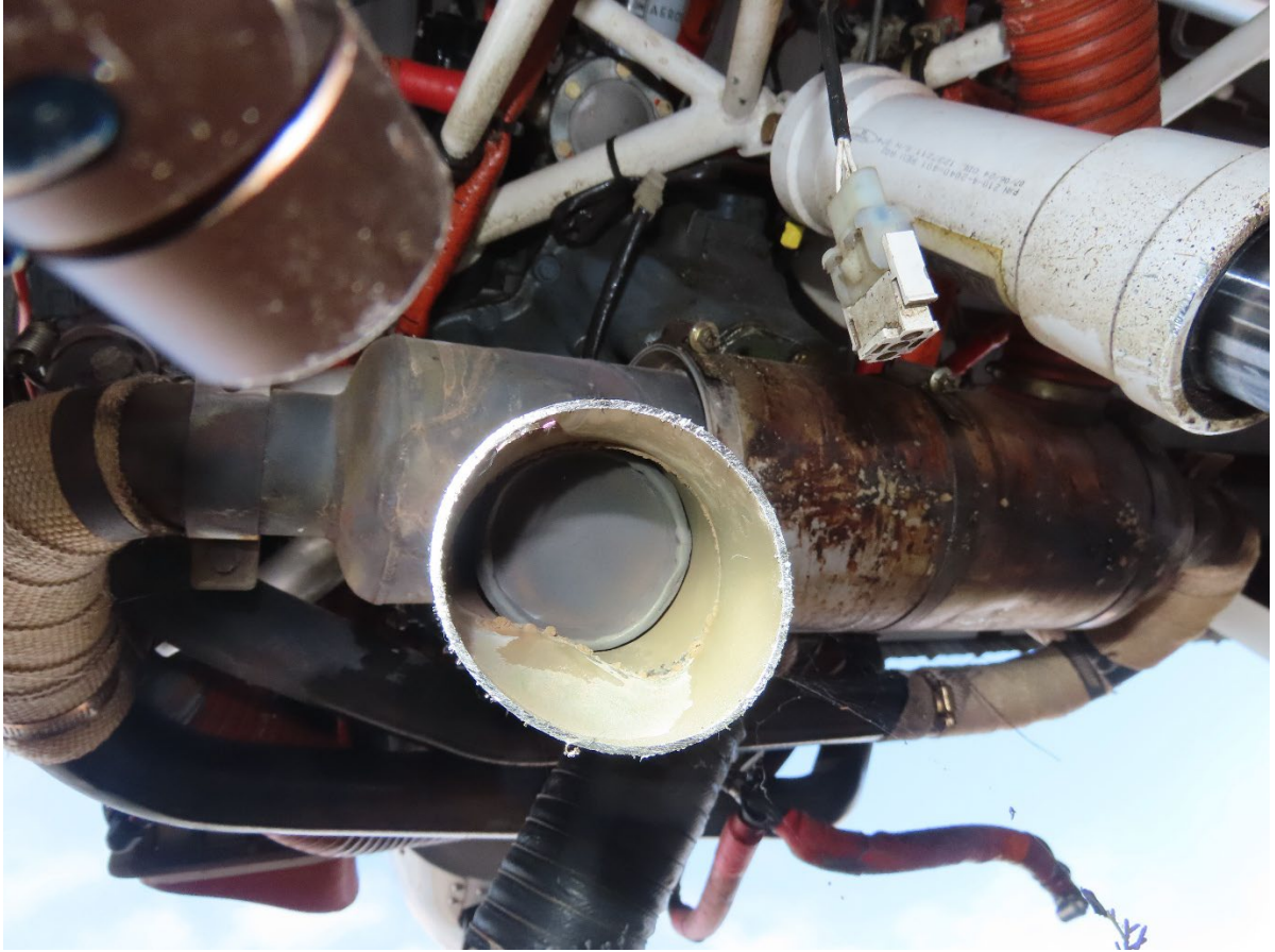
Figure 1. Blocked exhaust as found
