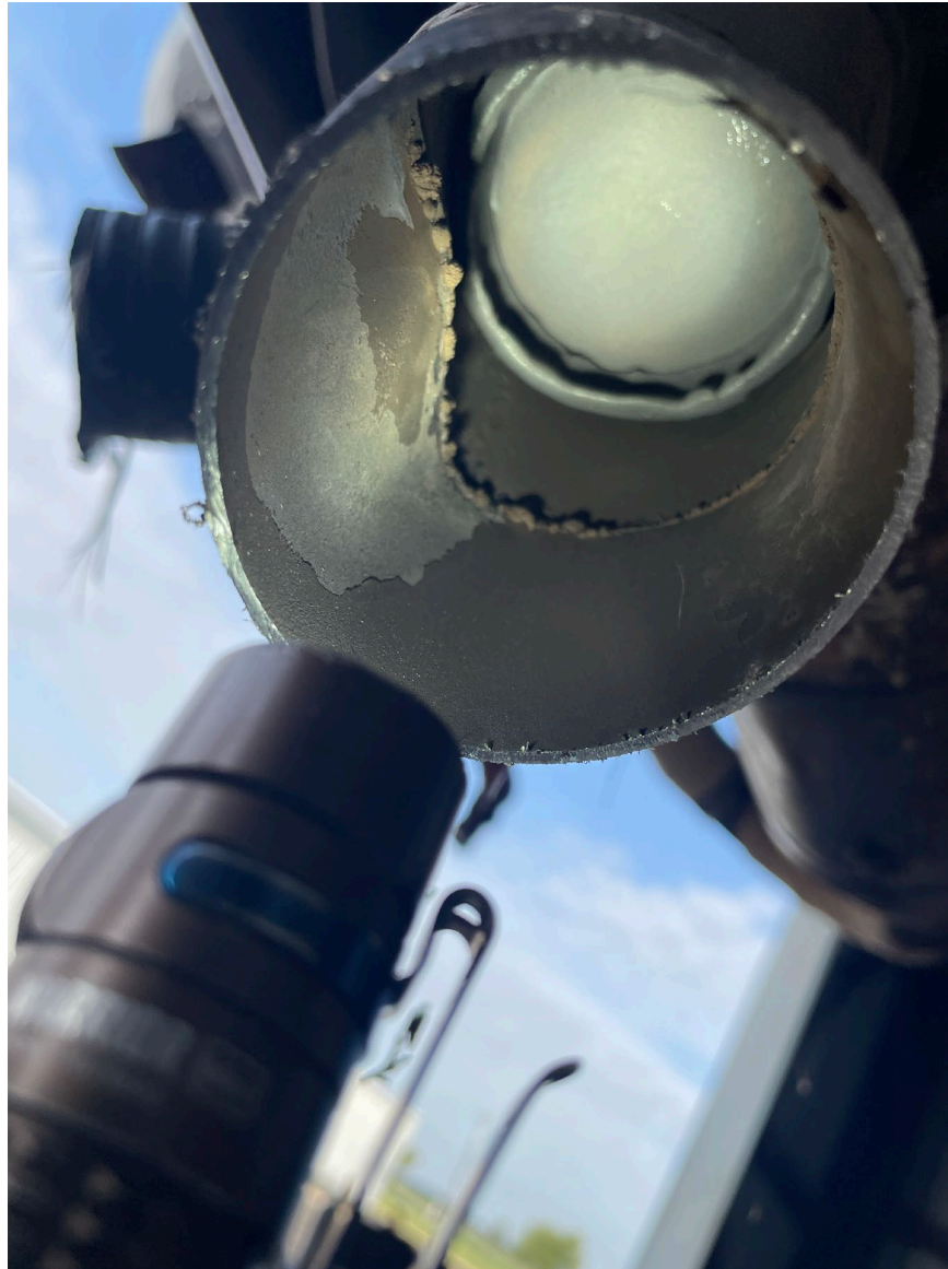
Photograph 3 - Engine exhaust blockage as found (NTSB Photo)
