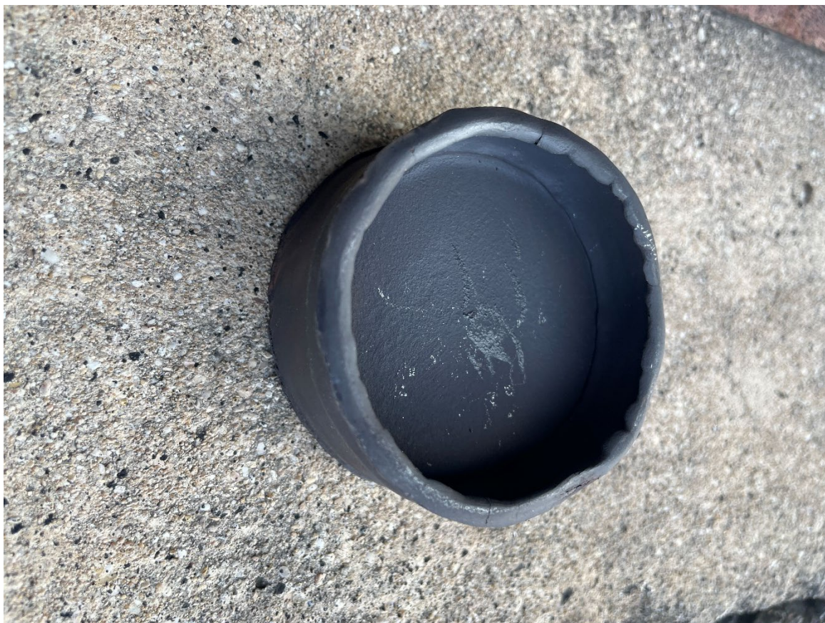
Photograph 4 - Steel baffle plate removed from tailpipe (NTSB Photo)
