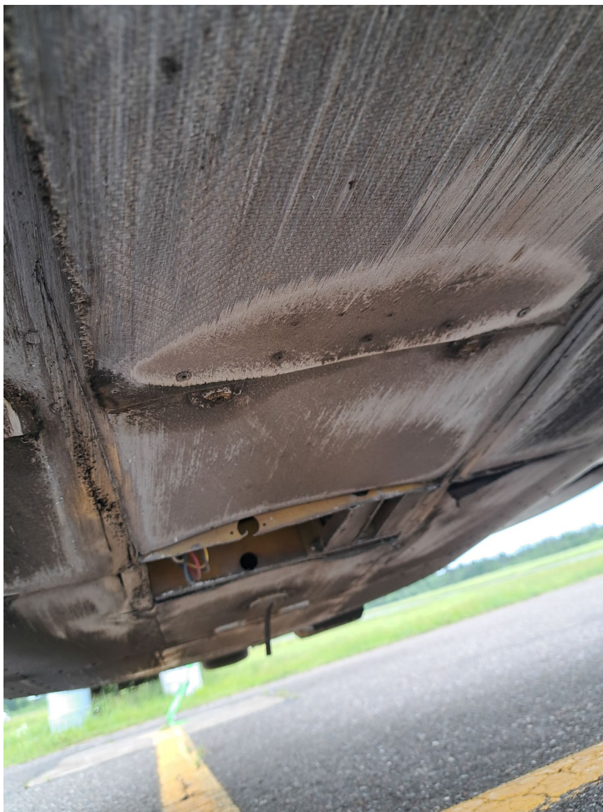
Photograph 1 - Damage to underside of fuselage (Courtesy of FAA)
