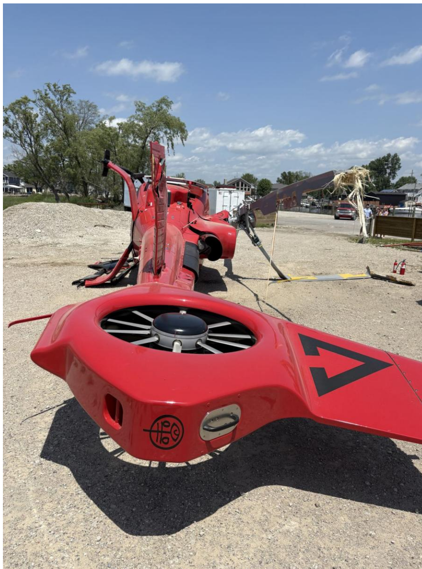
Photograph 4 - Fenestron and Tailboom (FAA Photo)
