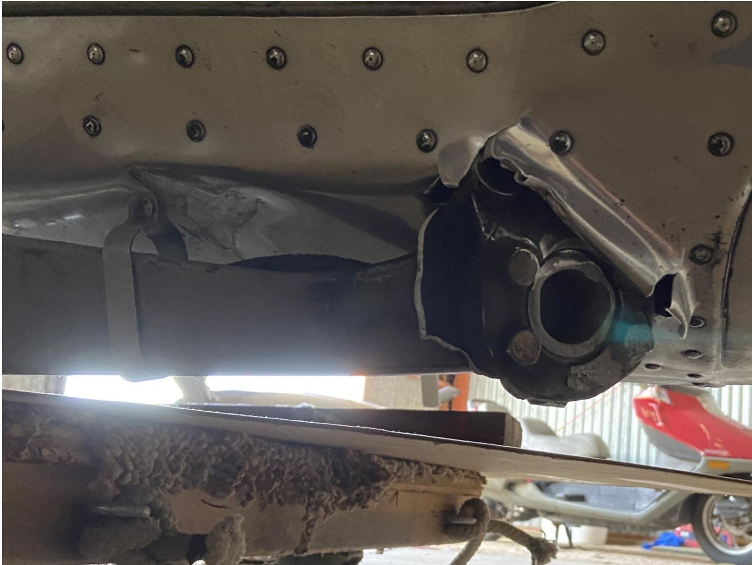
Photograph 5 - Fuselage Damage (Courtesy of FAA)
