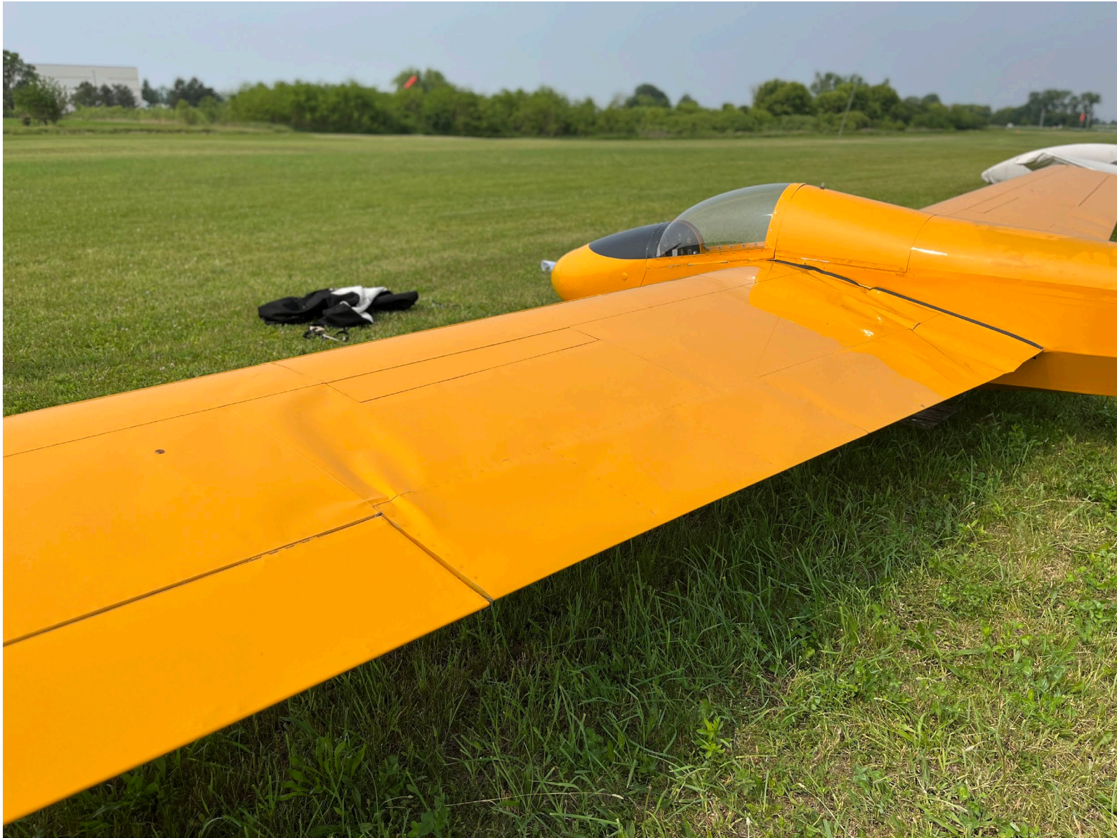
Photograph 2 - Left wing damage (Courtesy of FAA)
