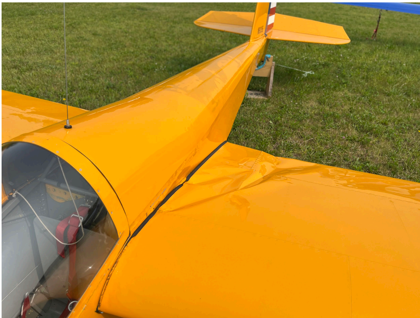
Photograph 3 - Inboard left wing damage (Courtesy of FAA)
