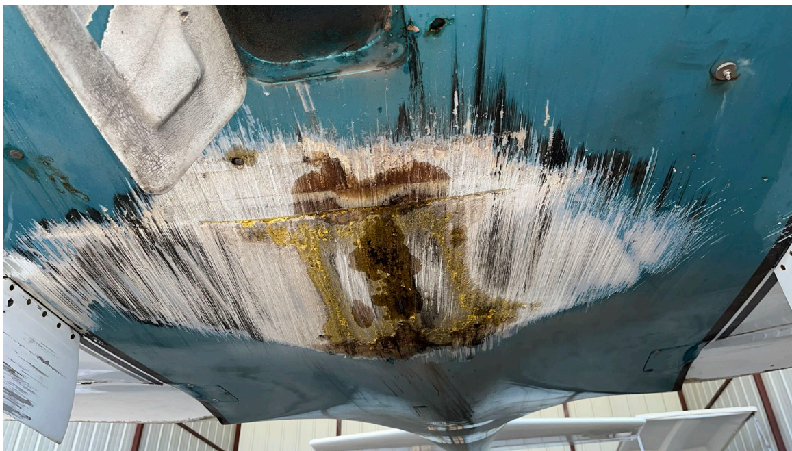
Photograph 1 - Accident airplane abrasion damage (Courtesy of FAA)
