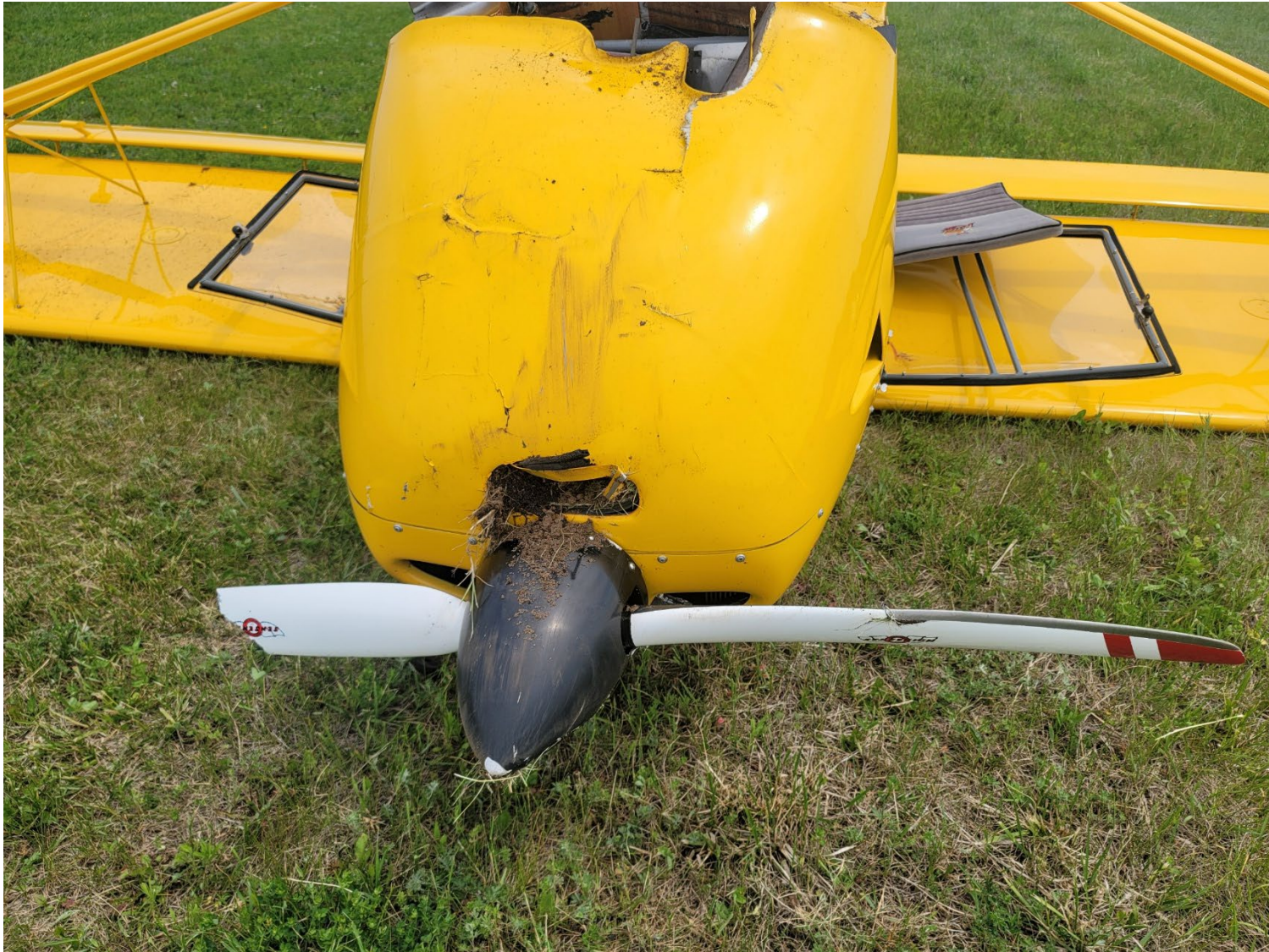
Photograph 3 - N755SD propeller & lower engine cowling (Courtesy of airport manager)
