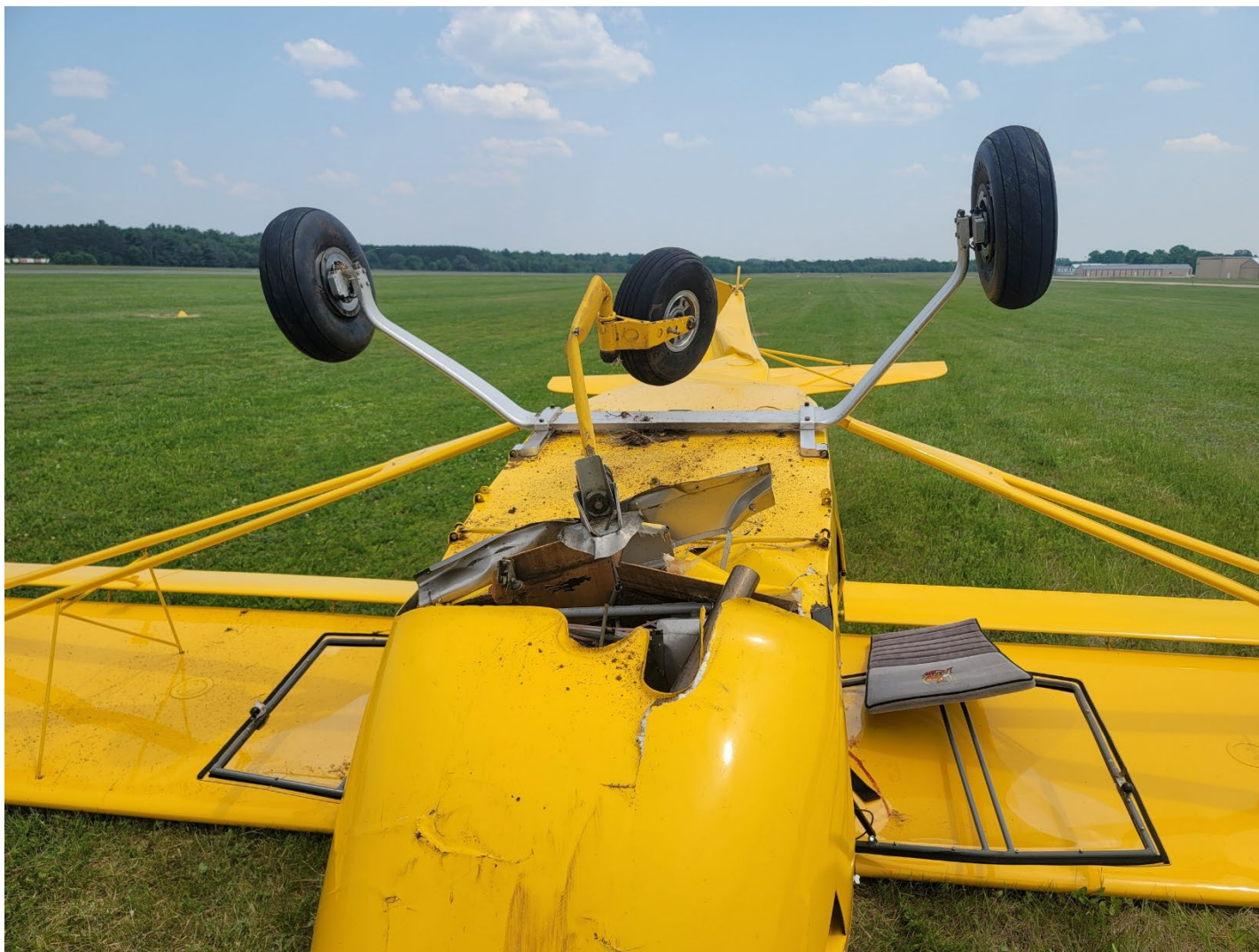
Photograph 4 - N755SD nose landing gear / belly damage (Courtesy of airport manager)
