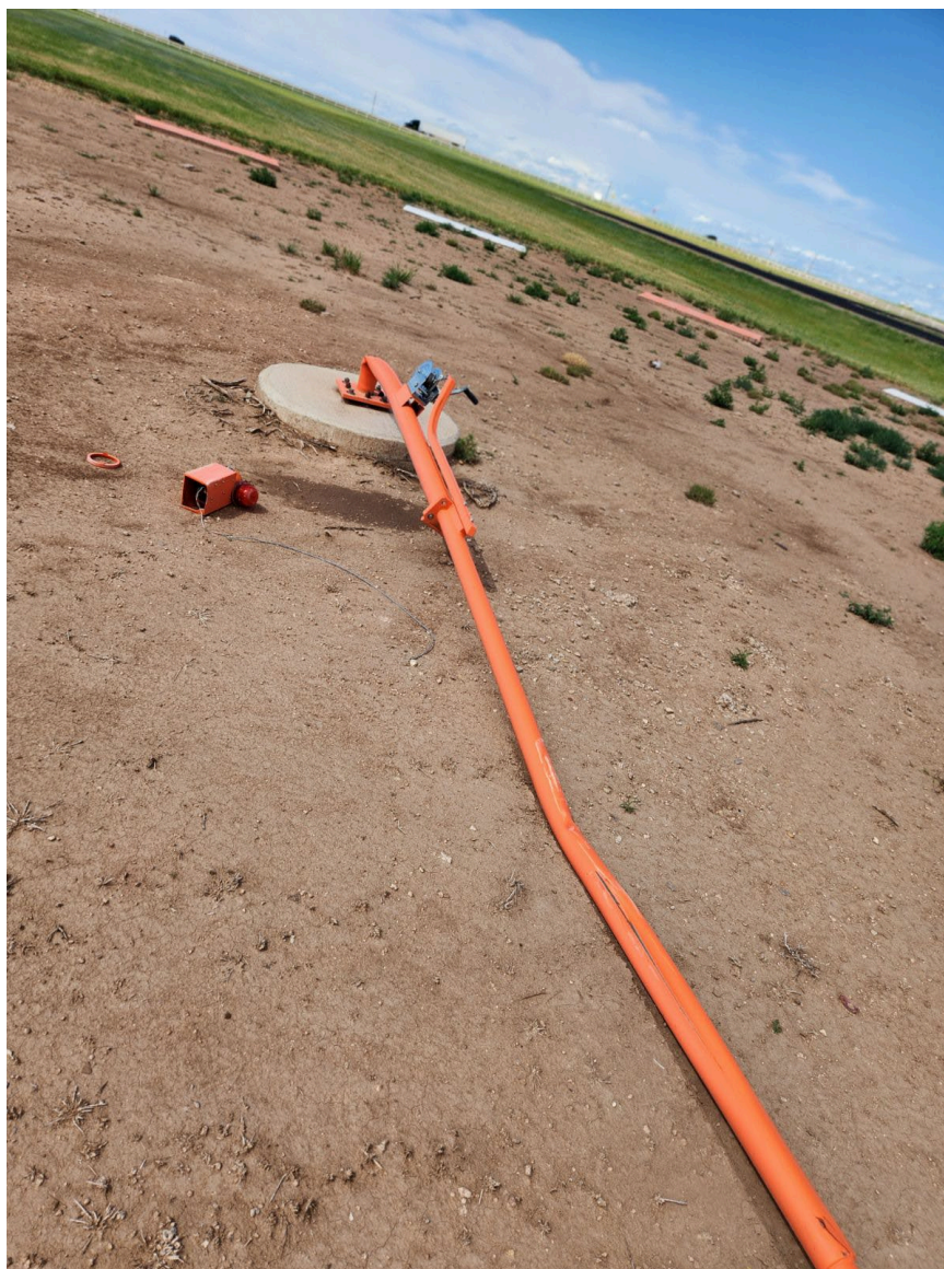
Photograph 1 - View of the wind cone that was impacted by the airplane (courtesy of the Texas Department of Public Safety)
