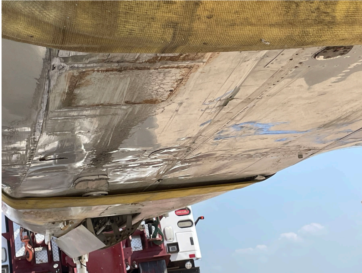
Photograph 1 - Abrasion damage (Courtesy of FAA)
