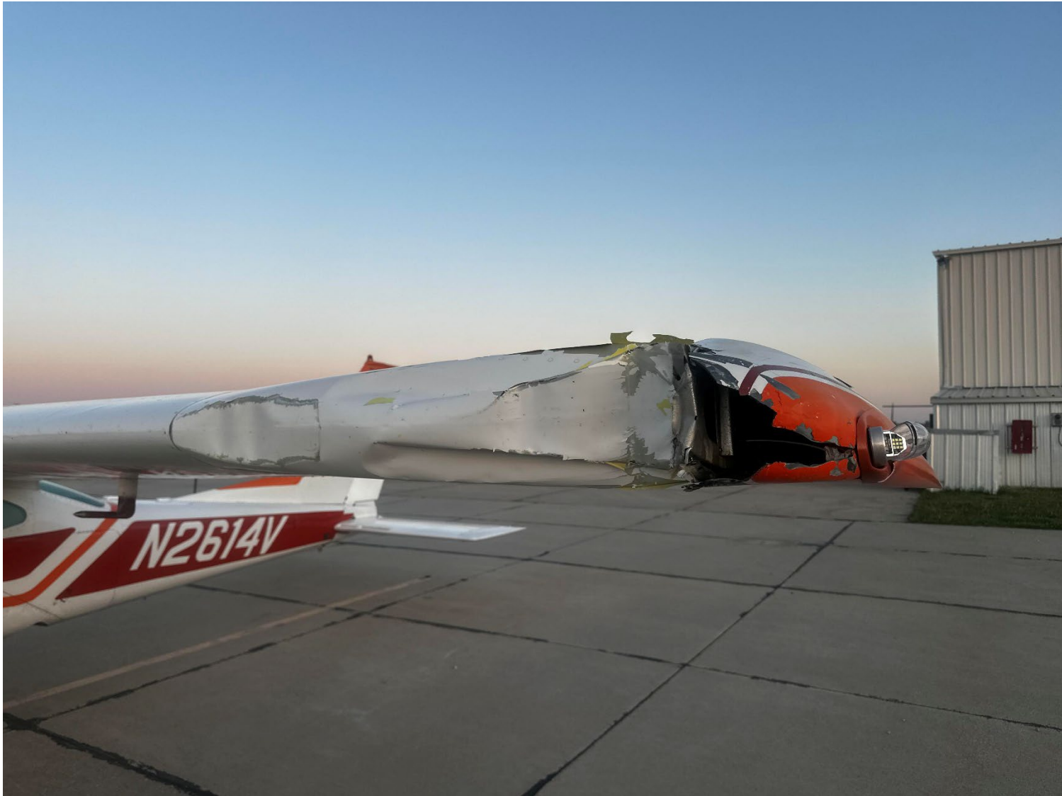
Photograph 1 - Damaged left wing (Courtesy of pilot)
