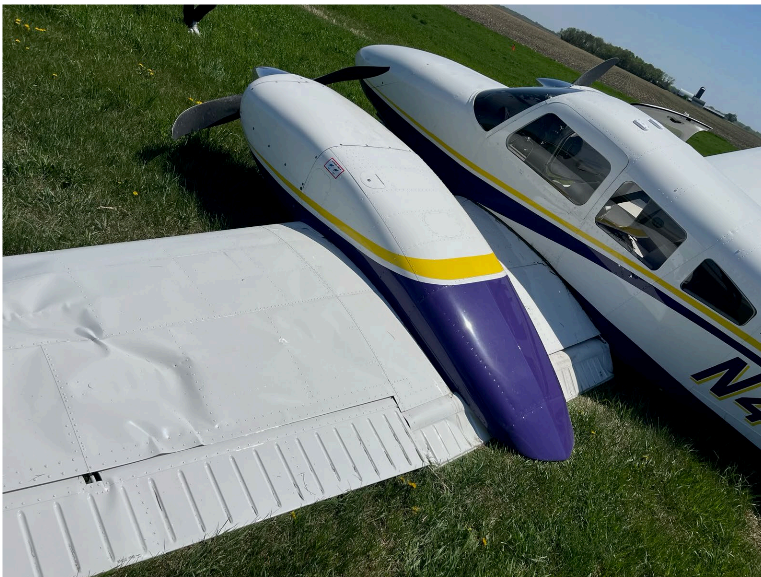
Photograph 3 - Left Wing Damage (Courtesy of Federal Aviation Administration)
