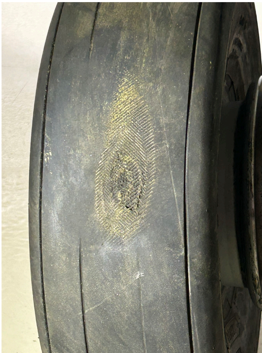
Photograph 2 - Worn Left Tire with Flat Spot (Courtesy of Federal Aviation Administration)
