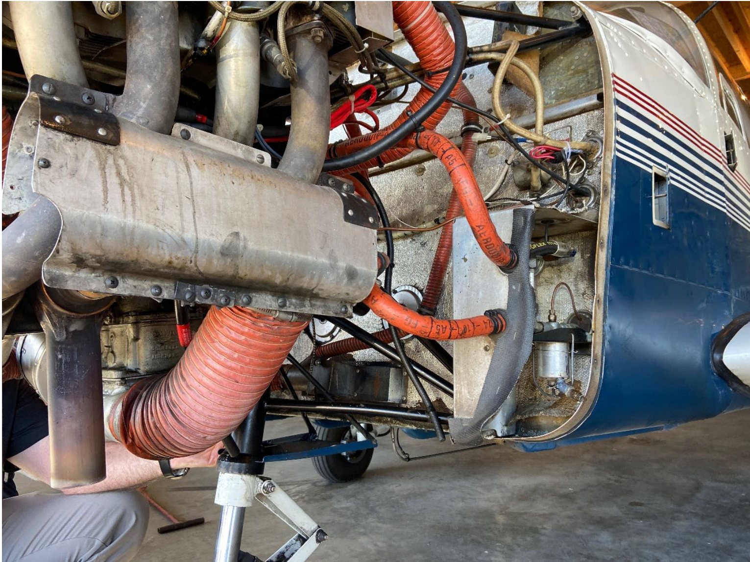
Photograph 1 - View of the bent engine mount (courtesy of the Federal Aviation Administration)
