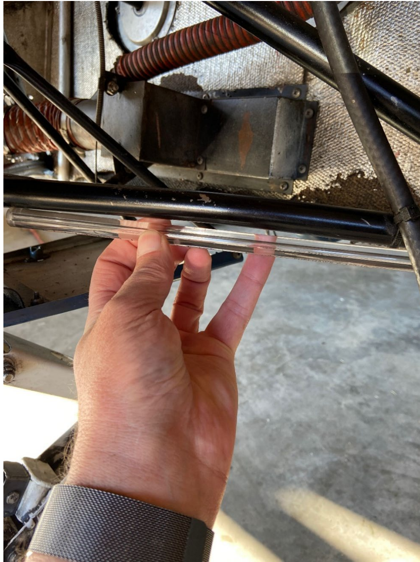
Photograph 3 - View of the bent engine mount (courtesy of the Federal Aviation Administration)
