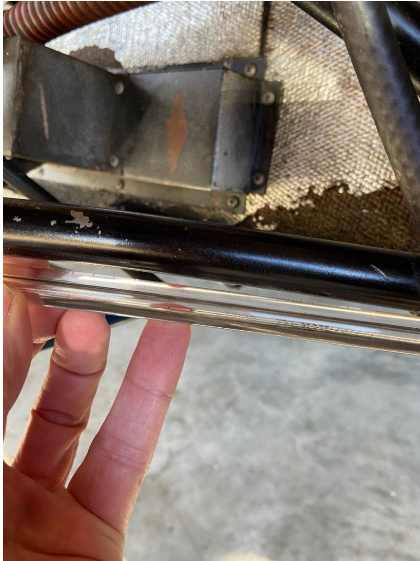
Photograph 4 - View of the bent engine mount (courtesy of the Federal Aviation Administration)
