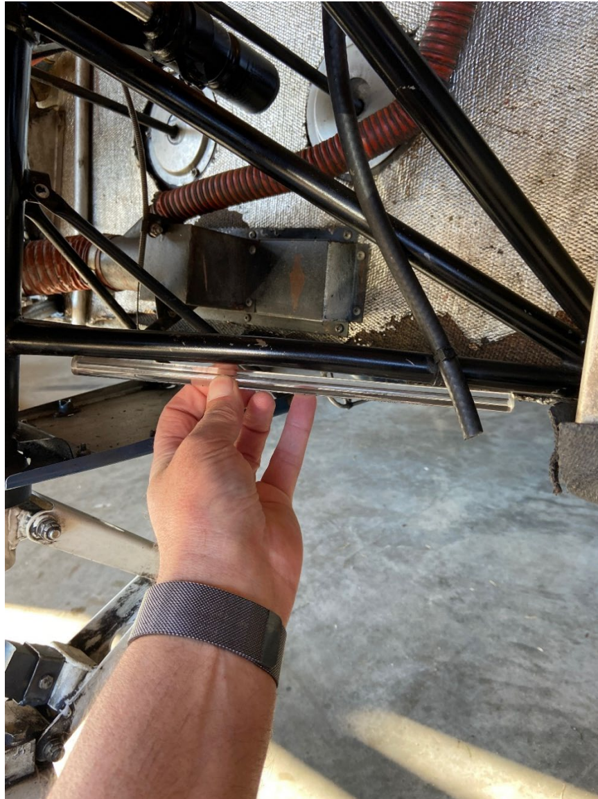
Photograph 2 - View of the bent engine mount (courtesy of the Federal Aviation Administration)
