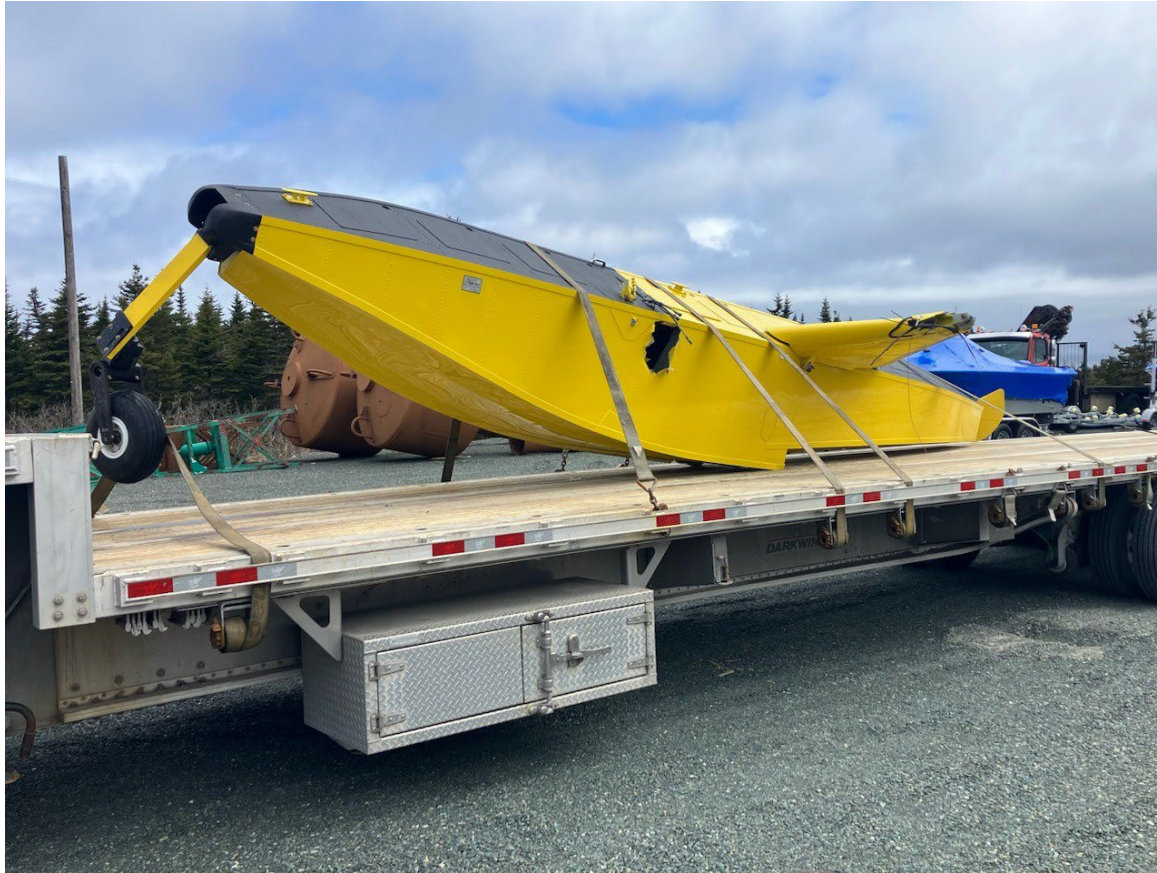
Photograph 5 - Recovered Right Pontoon (Courtesy of the Canadian Coast Guard)
