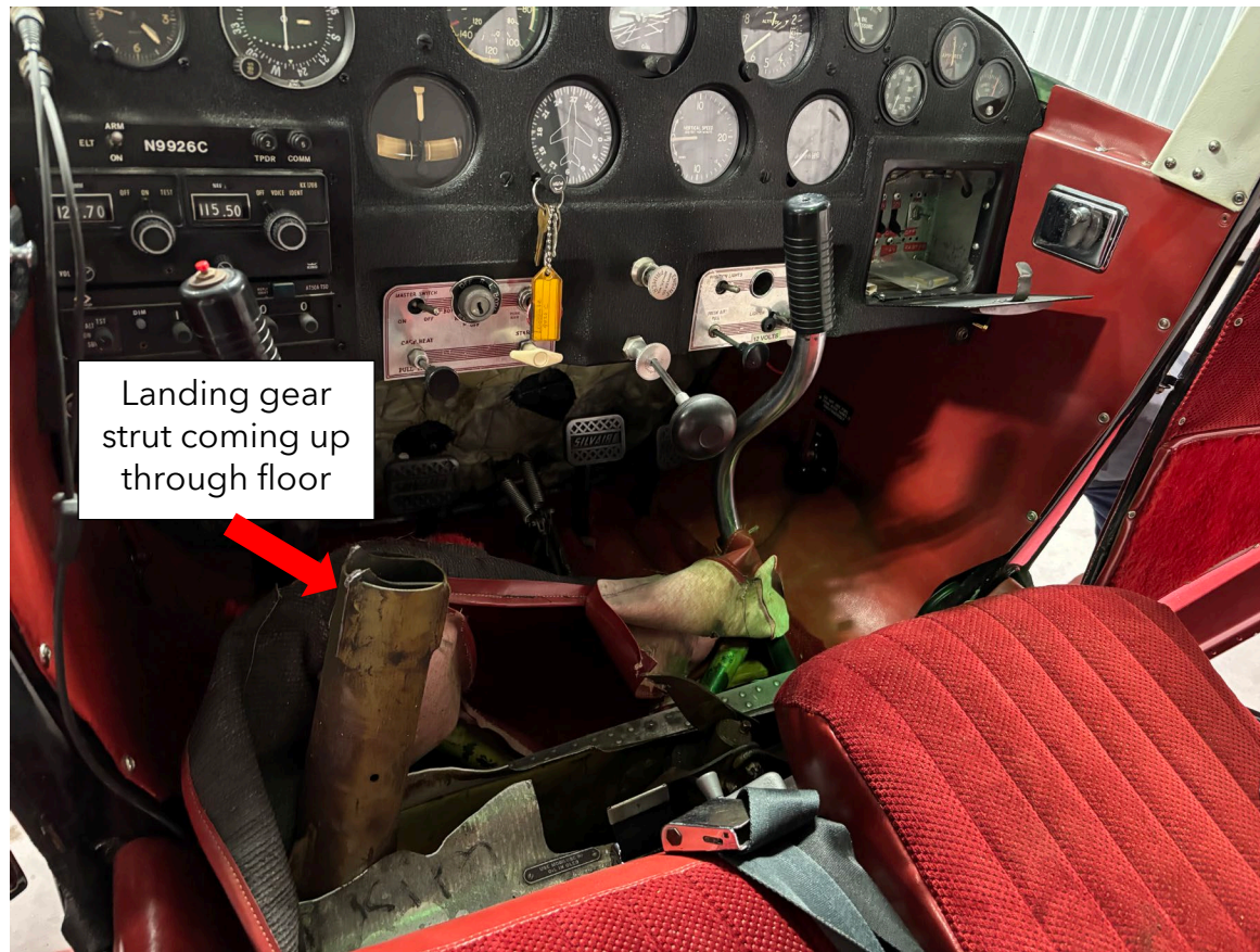
Photograph 2 - Landing gear penetration of floor (Courtesy of FAA)
