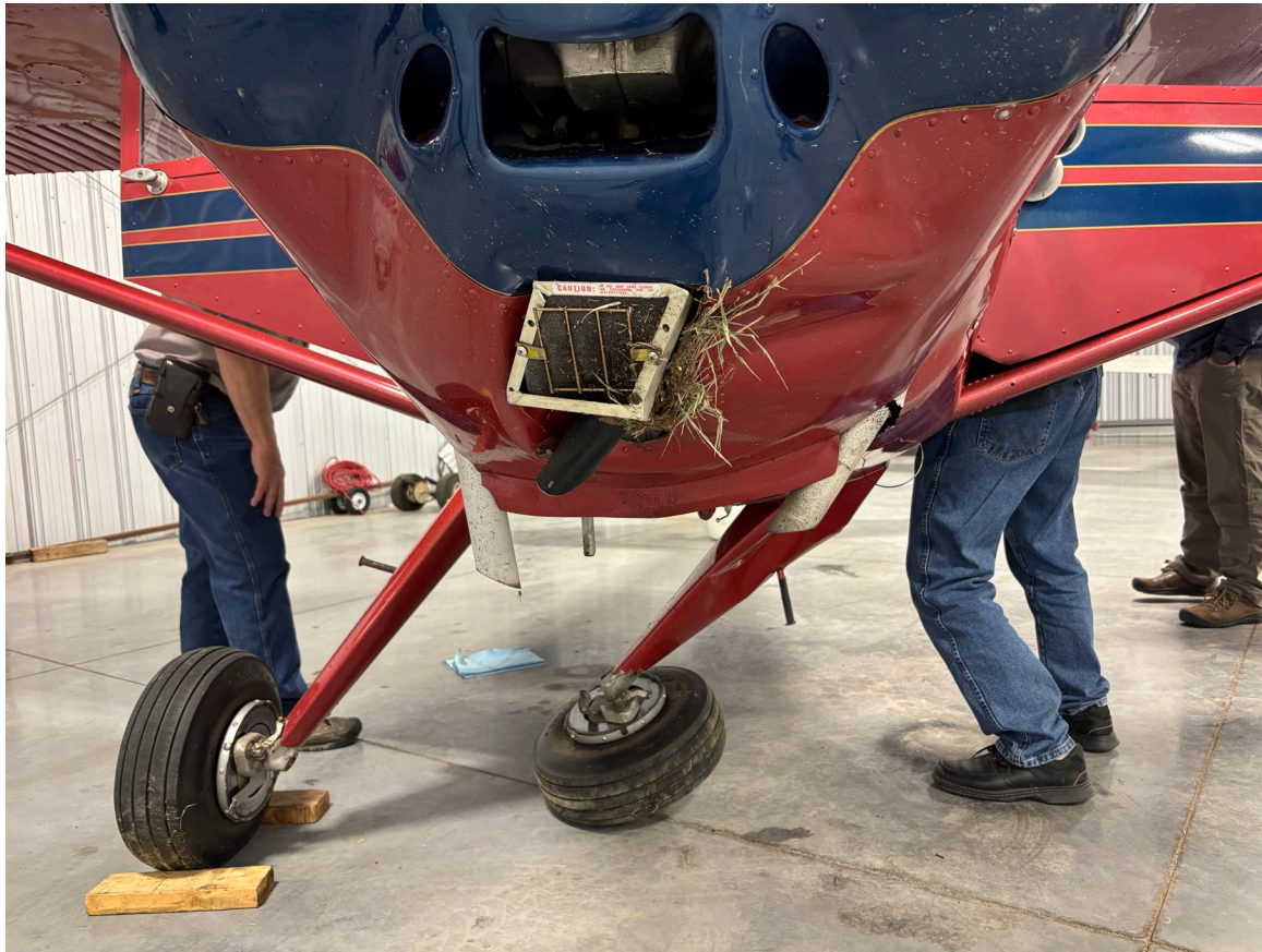
Photograph 1 - Wrinkling of lower fuselage (Courtesy of FAA)
