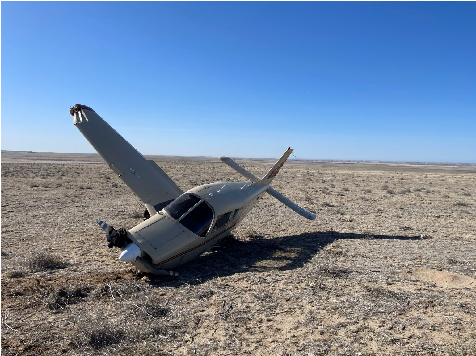
Photograph 1 - View of the front of the airplane at the accident site with the left wing separated (courtesy of the flight instructor)
