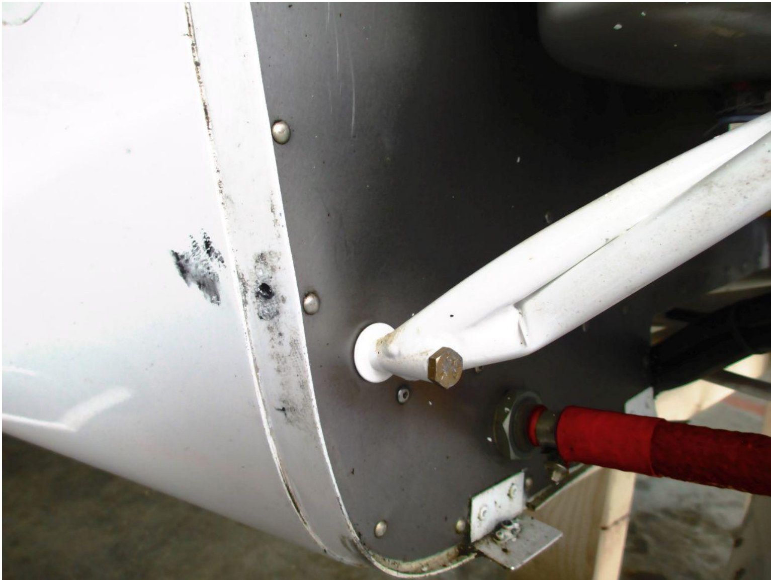
Photograph 5 - Engine Mount (FAA Photo)
