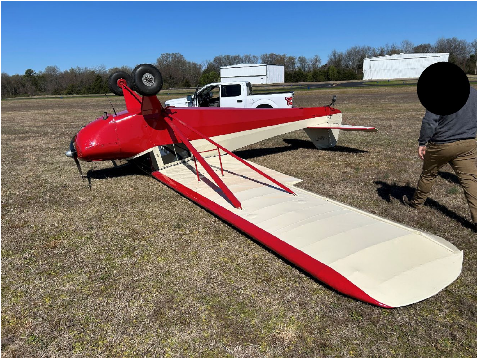
Photograph 8 - Side view of N39158 Taylorcraft BC-12D inverted on a grass field (courtesy of the N39158 pilot)
