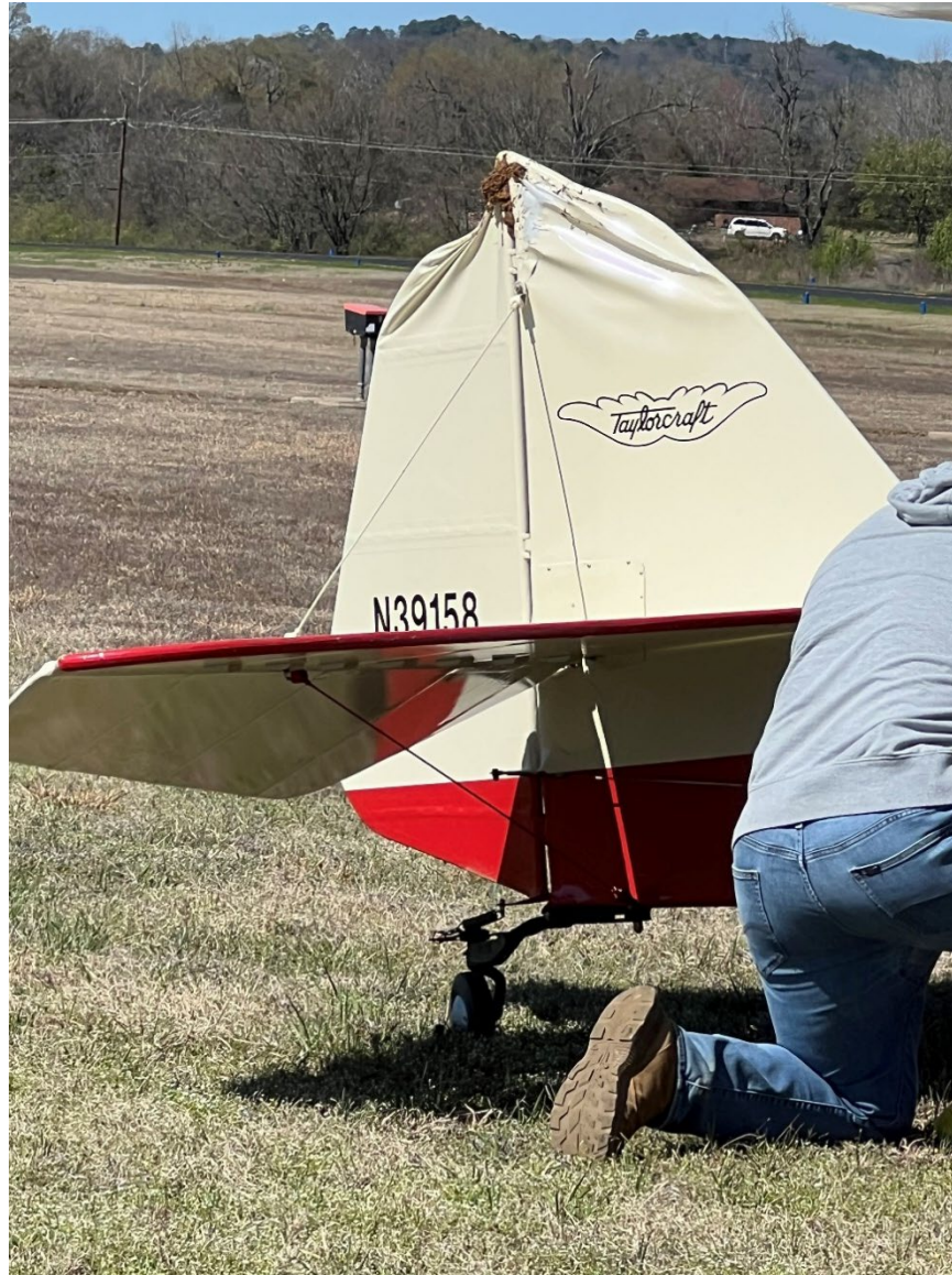
Photograph 11 - View of the substantial damage sustained to the empennage of N39158 Taylorcraft BC-12D (courtesy of the N39158 pilot)
