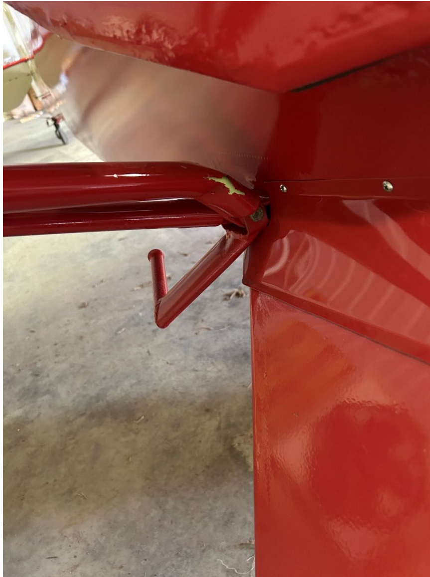
Photograph 12 - View of the substantial damage sustained to the right wing strut of N39158 Taylorcraft BC-12D (courtesy of the N39158 pilot)
