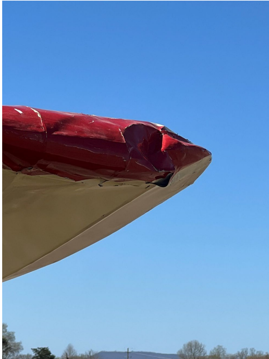
Photograph 10 - View of the substantial damage sustained to the left wing of N39158 Taylorcraft BC-12D (courtesy of the N39158 pilot)
