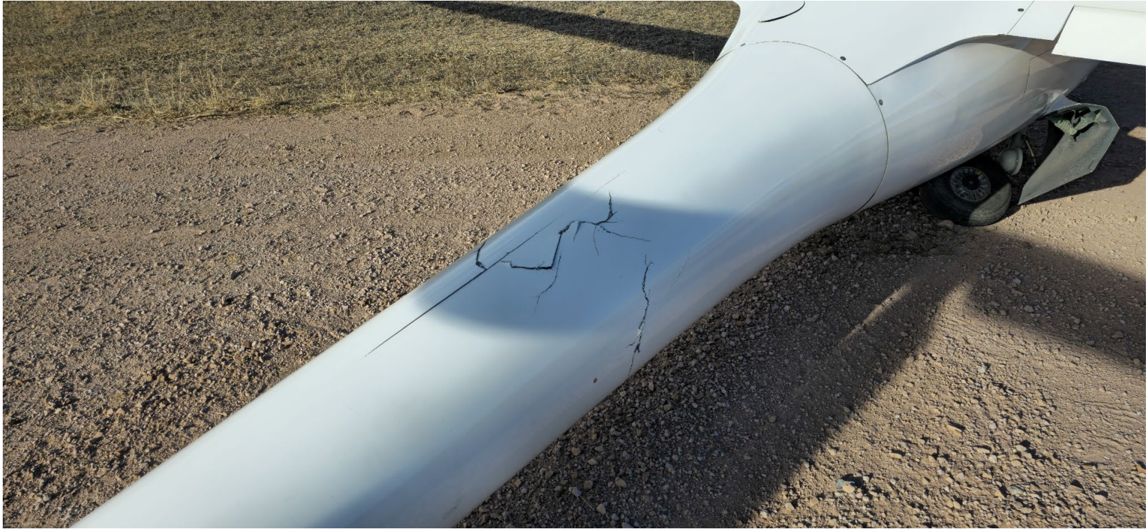
Photograph 2 - Substantial Fuselage Damage (Courtesy of Pilot)
