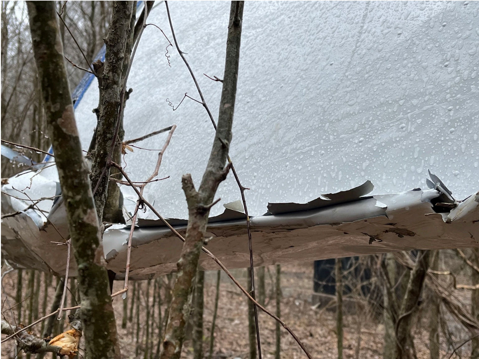
Photograph 2 - Right Wing Damage (Courtesy of Federal Aviation Administration)
