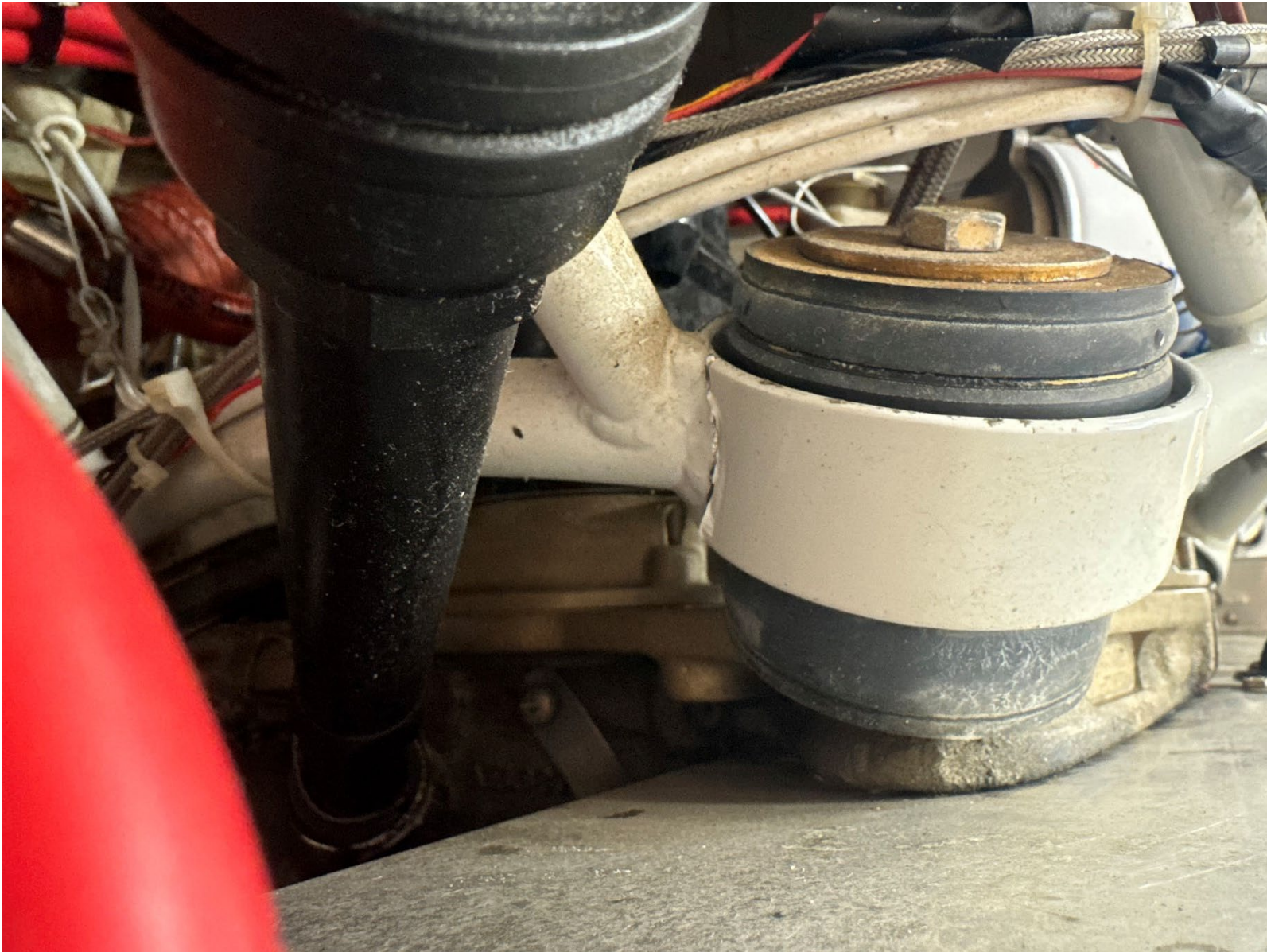
Photograph 3 - Broken engine mount (Courtesy of the Pilot/Owner)
