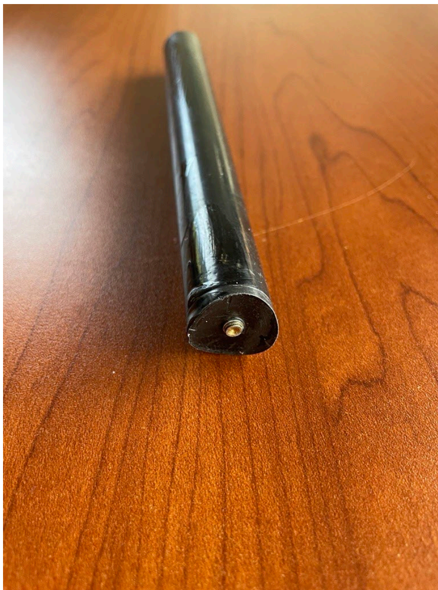
Photograph 1 - Separated Anchor Point (Courtesy of NTSB)
