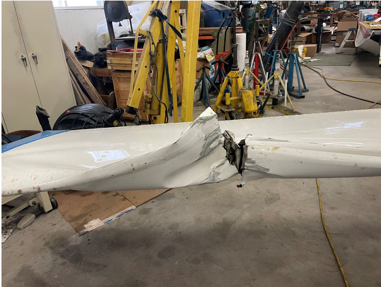
Photograph 1 - Damage to Left Stabilator (Courtesy of Pilot)
