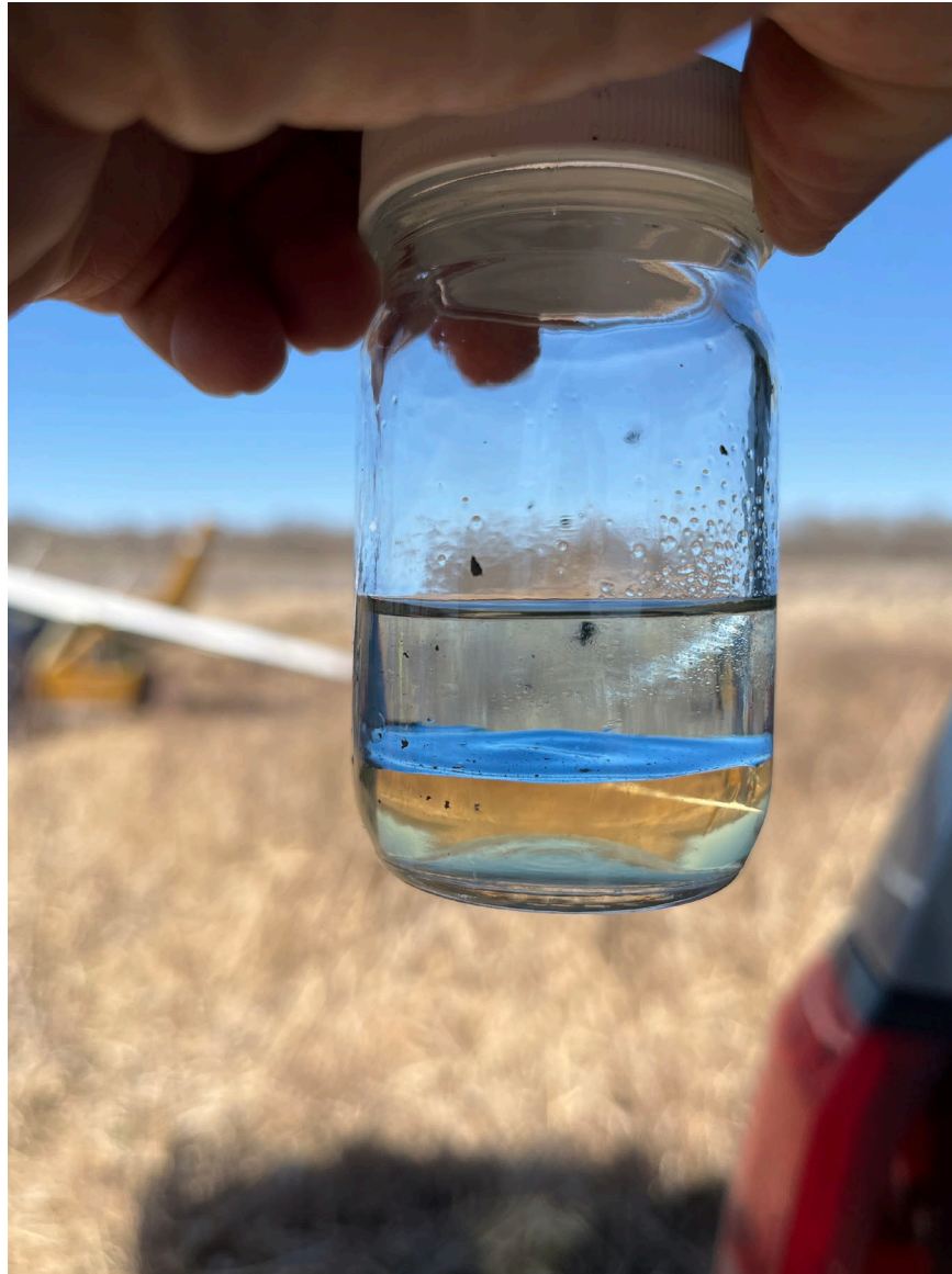
Photograph 3 - Fuel sample from inline strainer (Courtesy of FAA)
