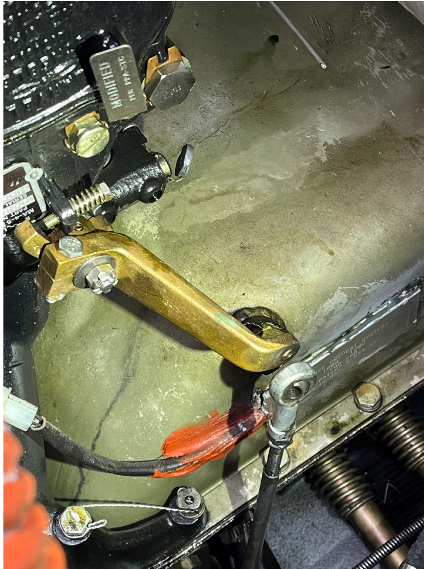
Photograph 2 - Throttle Arm and Cable End (Courtesy of FAA)
