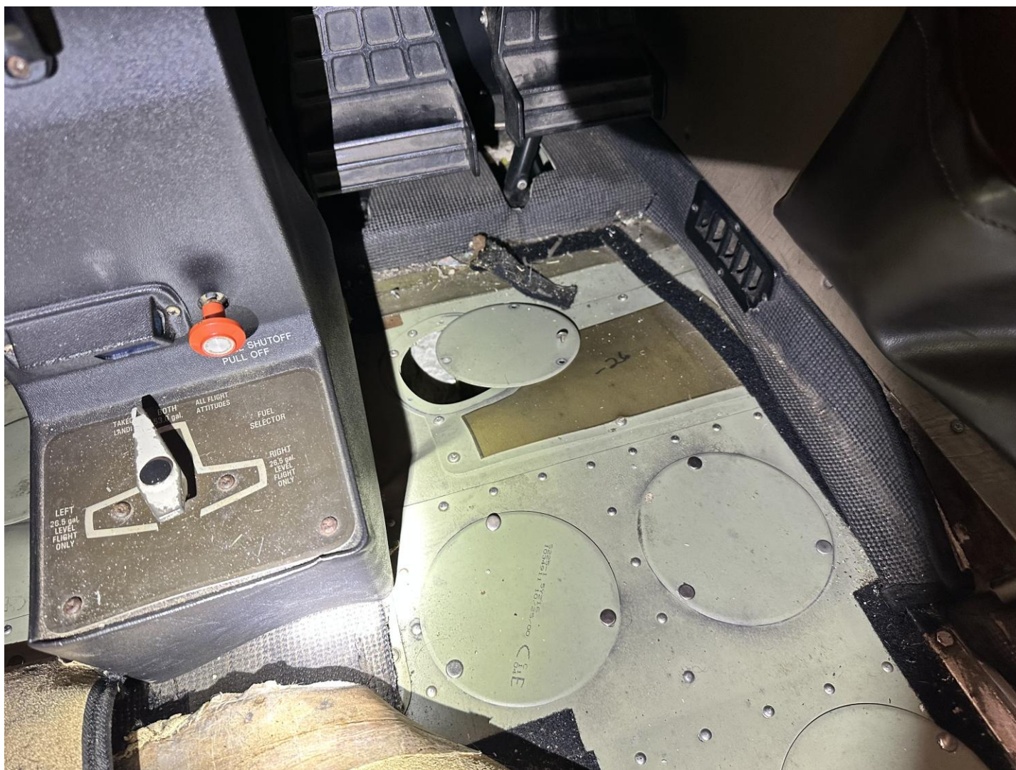
Photograph 3 - Lower Airframe Damage, Right Pilot Position (Courtesy of FAA)
