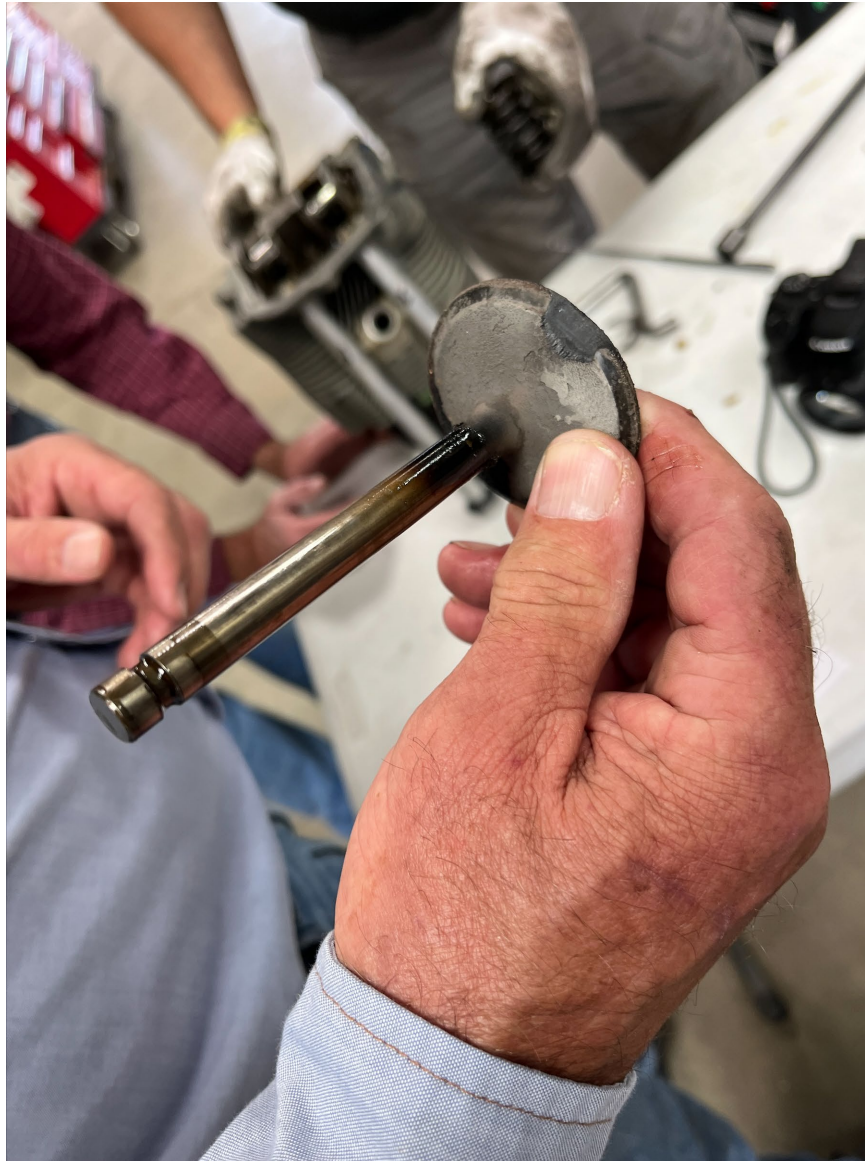
Photograph 3 - Damaged Number 3 Cylinder Intake Valve (Courtesy of FAA)
