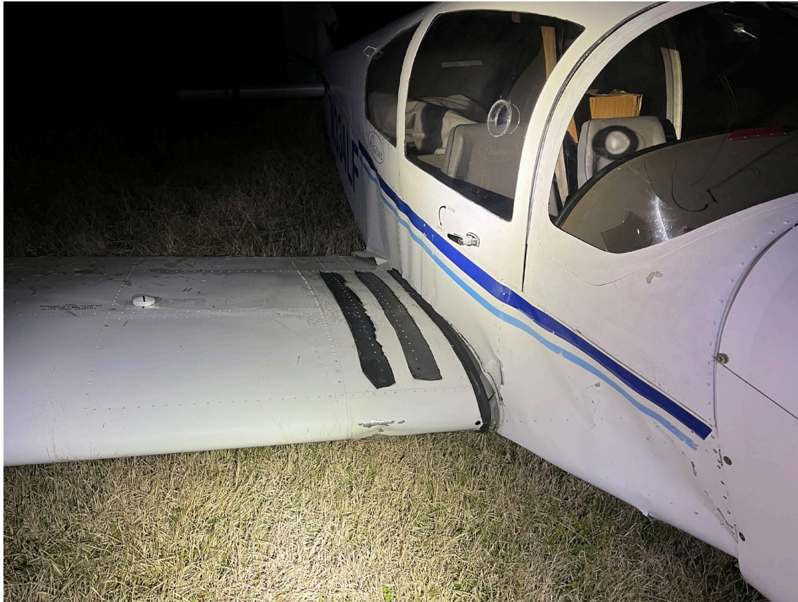
Photograph 2 - Substantial Damage to Fuselage (Courtesy of FAA)
