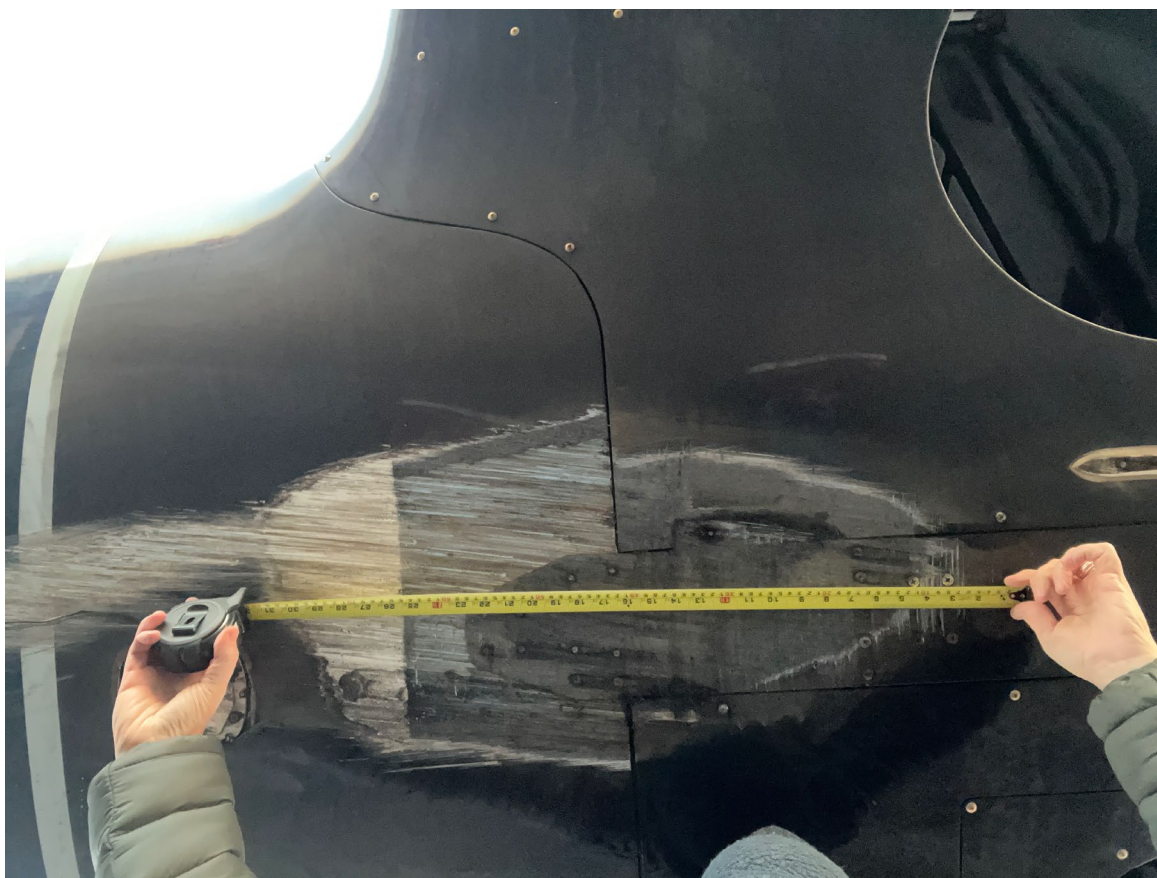
Photograph 3 - Damage to airplane (Courtesy of FAA)
