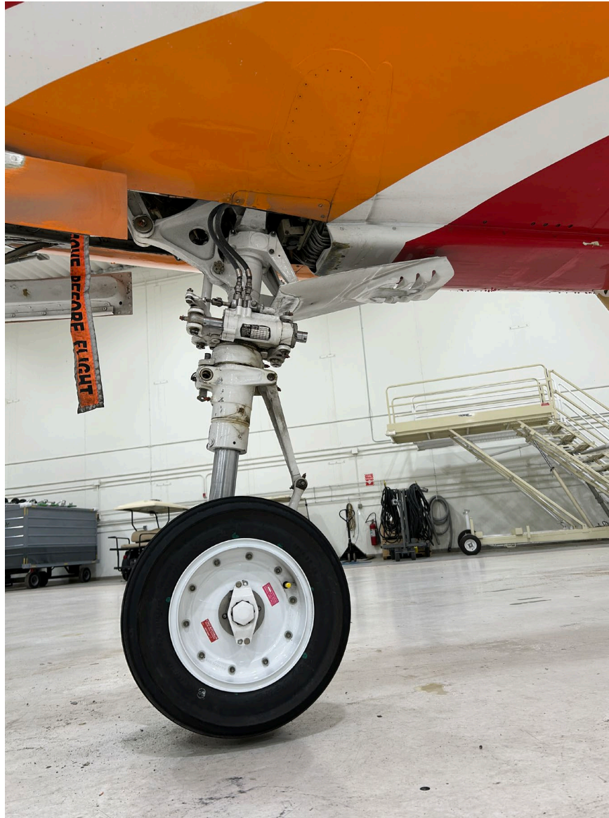
Photograph 1 - Nose Landing Gear Fully Extended and Locked Down (Courtesy of FAA)
