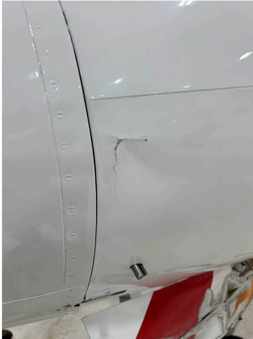
Photograph 2 - Substantial Damage to Fuselage (Courtesy of FAA)
