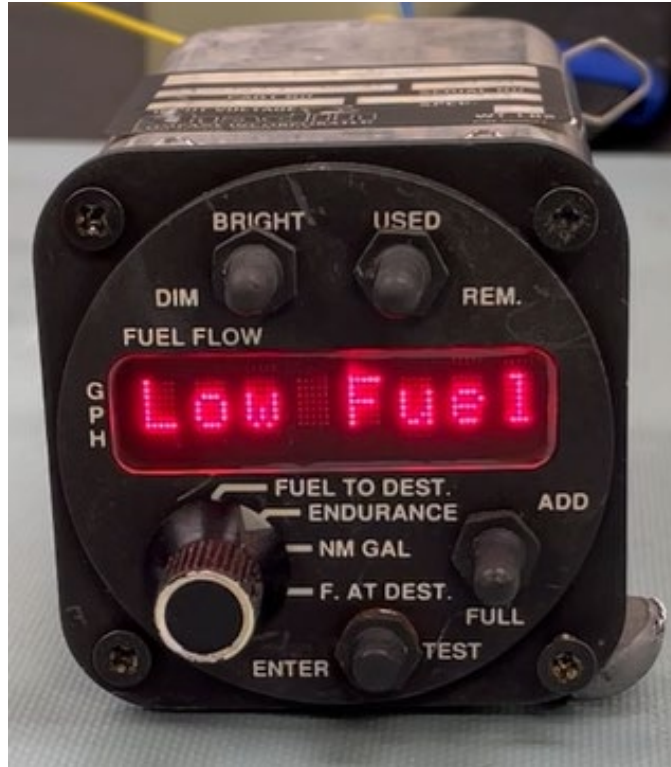
Figure 2. Shadin Microflo-L Low Fuel warning upon power up.
