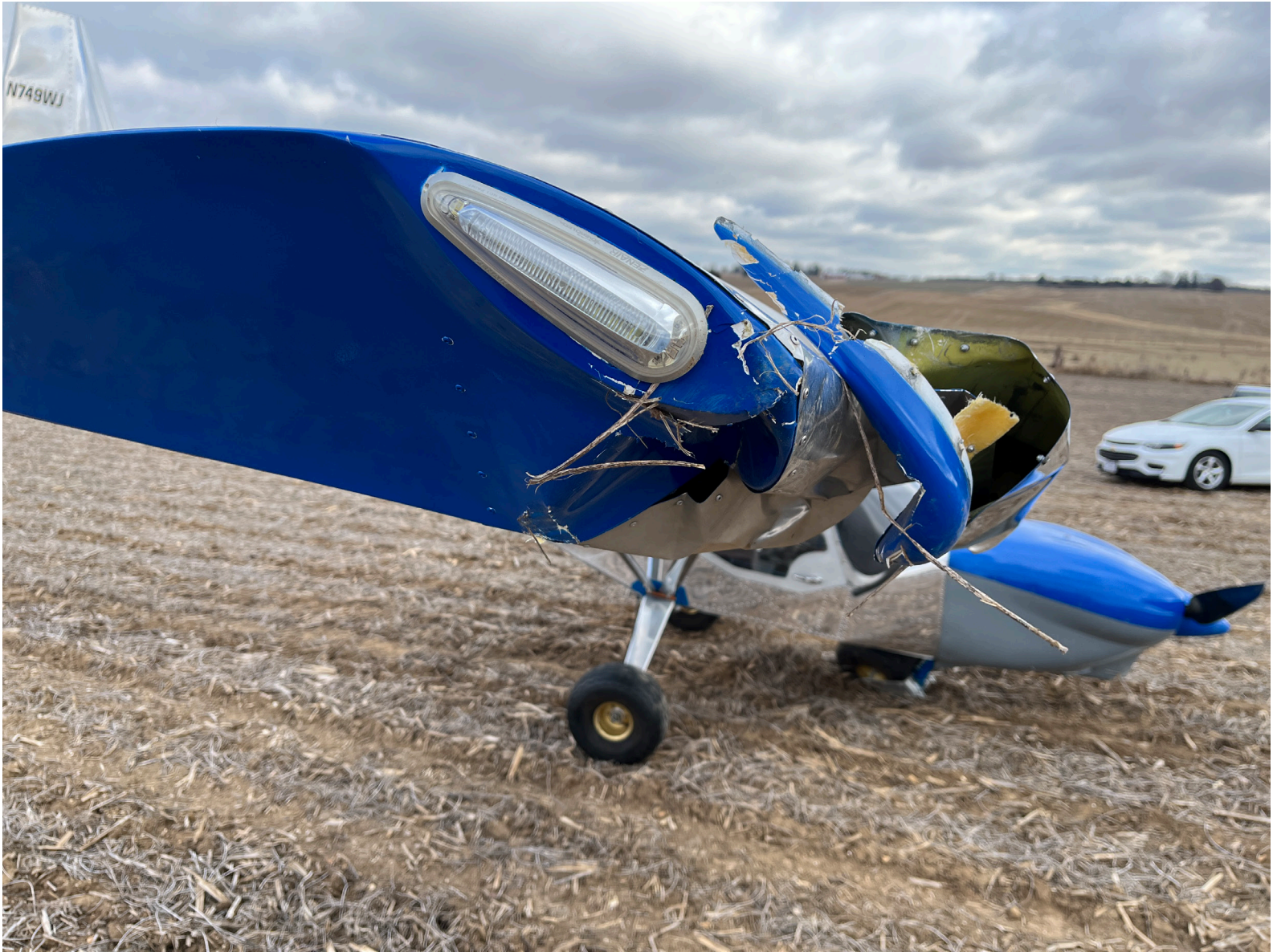
Photograph 3 - Right wing damage (Courtesy of FAA)
